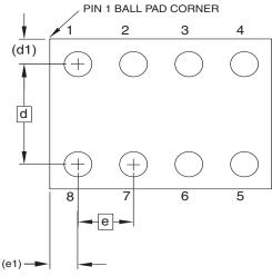
1. Dimension "b" is measured at the maximum solder ball diameter.
