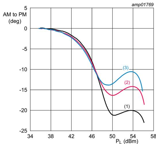
$V_{DS} = 30\text{ V}$ ;  $I_{Dq} = 770\text{ mA}$ ;  $V_{GS(amp)peak} = 0.764\text{ V}$ .
