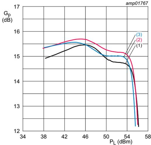
$V_{DS} = 30\text{ V}$ ;  $I_{Dq} = 650\text{ mA}$ ;  $V_{GS(amp)peak} = 0.745\text{ V}$ ;
