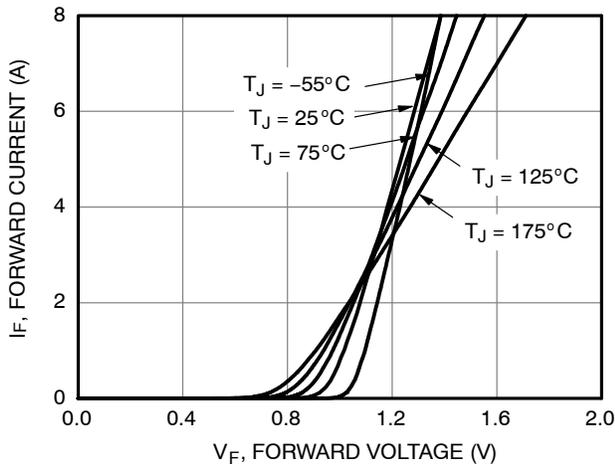
Figure 1. Forward Characteristics
