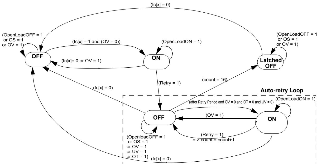
Figure 16. State Machine: Fault Occurrence and Auto-retry
