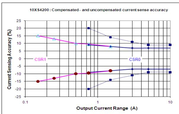
Figure 18. Current Sense Accuracy Versus Output Current
