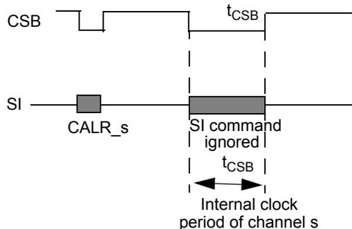
When the duration of the negative CSB pulse is outside a predefined time slot (from  $t_{CSB(MIN)}$  to  $t_{CSB(MAX)}$ ), the calibration event is ignored and the internal clock frequency remains unchanged. If the value ( $f_{PWM(0)}$ ) has not been previously calibrated, it remains at its default level.
