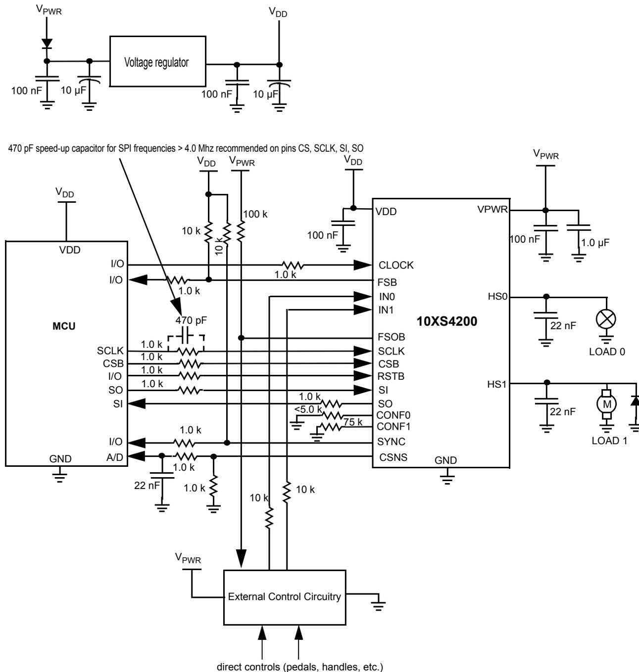
Figure 21. Typical Application with Two Different Load Types
