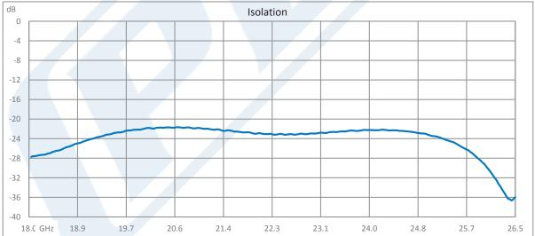
Click the following link (or enter part number in "SEARCH" on website) to obtain additional part information including price, inventory and certifications: High Power Circulator With 17 dB Isolation From 18 GHz to 26.5 GHz, 50 Watts And SMA Female PE83CR1012
