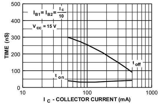
Figure 8. Turn-On and Turn-Off Times vs. Collector Current
