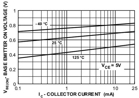
Figure 4. Base-Emitter On Voltage vs. Collector Current
