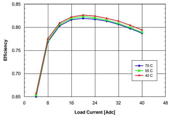
Figure 1.0V.12. Efficiency vs. load current and ambient temperature for QME48T40010 converter mounted horizontally with  $V_{in} = 48\text{ V}$  and air flowing from pin 1 to pin 3 at a rate of 200 LFM (1.0 m/s).
