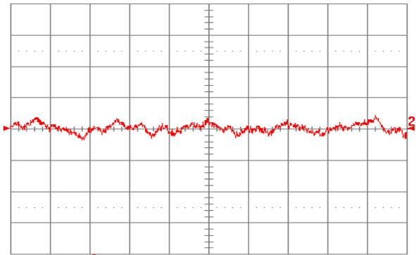
Figure 2.5V.22. Input reflected ripple current,  $i_s$  (10 mA/div.), measured through 10  $\mu\text{H}$  at the source at full rated load current and  $V_{in} = 48 \text{ V}$ . Refer to Fig. 2.5V.20 for test setup. Time scale: 1  $\mu\text{s}/\text{div}$ .
