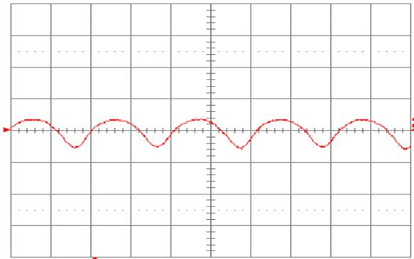
Figure 1.0V.21. Input reflected ripple current,  $i_c$  (100 mA/div.), measured at input terminals at full rated load current and  $V_{in} = 48 \text{ V}$ . Refer to Fig. 1.0V.20 for test setup. Time scale:  $1 \mu\text{s}/\text{div}$ .
