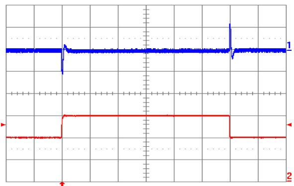
Figure 1.5V.18. Output voltage response to load current step-change (20 A – 30 A – 20 A) at  $V_{in} = 48\text{ V}$ . Top trace: output voltage (100 mV/div.). Bottom trace: load current (10 A/div.). Current slew rate: 5A/ $\mu\text{s}$ .  $C_o = 470\ \mu\text{F POS} + 1\ \mu\text{F}$  ceramic. Time scale: 0.2 ms/div.
