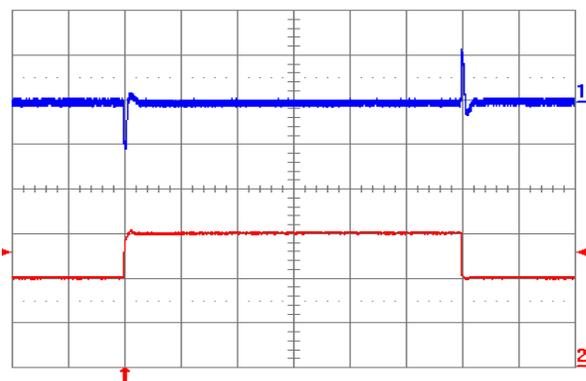
Figure 1.2V.18. Output voltage response to load current step-change (20 A – 30 A – 20 A) at  $V_{in} = 48\text{ V}$ . Top trace: output voltage (100 mV/div.). Bottom trace: load current (10 A/div.). Current slew rate: 5 A/ $\mu\text{s}$ .  $C_o = 470\ \mu\text{F}$  POS + 1  $\mu\text{F}$  ceramic. Time scale: 0.2 ms/div.
