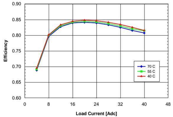
Figure 1.2V.12. Efficiency vs. load current and ambient temperature for QME48T40012 converter mounted horizontally with  $V_{in} = 48\text{ V}$  and air flowing from pin 1 to pin 3 at a rate of 200 LFM (1.0 m/s).
