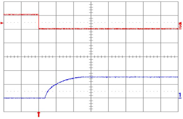
Figure 1.5V.16. Turn-on transient at full rated load current (resistive) plus 10,000  $\mu\text{F}$  at  $V_{in} = 48\text{ V}$ , triggered via ON/OFF pin. Top trace: ON/OFF signal (5 V/div.). Bottom trace: output voltage (1 V/div.). Time scale: 2 ms/div.
