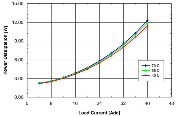
Figure 1.5V.14. Power dissipation vs. load current and ambient temperature for QME48T40015 converter mounted horizontally with  $V_{in} = 48\text{ V}$  and air flowing from pin 1 to pin 3 at a rate of 200 LFM (1.0 m/s).
