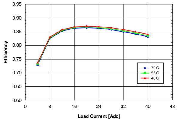
Figure 1.5V.12. Efficiency vs. load current and ambient temperature for QME48T40015 converter mounted horizontally with  $V_{in} = 48$  V and air flowing from pin 1 to pin 3 at a rate of 200 LFM (1.0 m/s).
