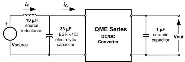
Figure 1.8V.20. Test setup for measuring input reflected ripple currents,  $i_c$  and  $i_s$ .
