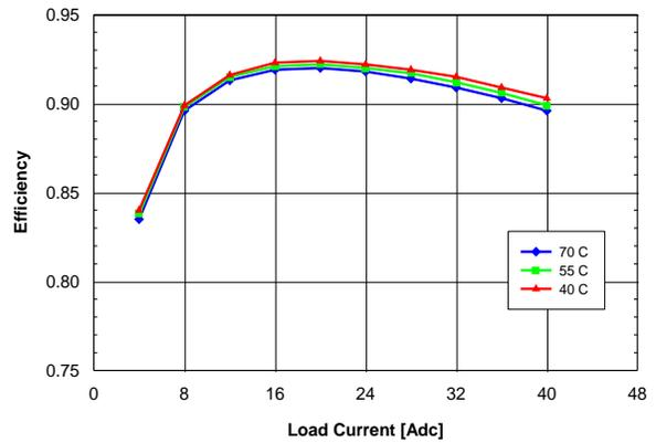
Figure 3.3V.12. Efficiency vs. load current and ambient temperature for QME48T40033 converter mounted horizontally with  $V_{in} = 48\text{ V}$  and air flowing from pin 1 to pin 3 at a rate of 200 LFM (1.0 m/s).
