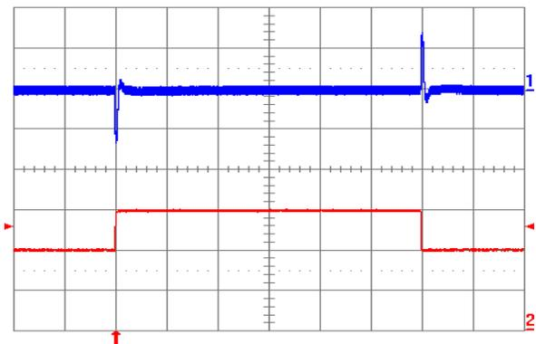
Figure 2.5V.18. Output voltage response to load current step-change (20 A – 30 A – 20 A) at  $V_{in} = 48\text{ V}$ . Top trace: output voltage (100 mV/div.). Bottom trace: load current (10 A/div.). Current slew rate: 5A/ $\mu\text{s}$ .  $C_o = 470\ \mu\text{F POS} + 1\ \mu\text{F}$  ceramic. Time scale: 0.2 ms/div.
