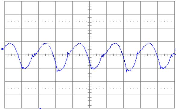
Figure 1.5V.19. Output voltage ripple (20 mV/div.) at full rated load current into a resistive load with  $C_o = 10 \mu\text{F}$  tantalum +  $1 \mu\text{F}$  ceramic and  $V_{in} = 48 \text{ V}$ . Time scale:  $1 \mu\text{s}/\text{div}$ .
