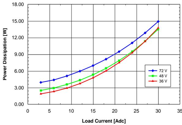
Figure 3.3V.13. Power dissipation vs. load current and input voltage for QME48T40033 converter mounted horizontally with air flowing from pin 1 to pin 3 at a rate of 300 LFM (1.5 m/s) and  $T_a = 25^\circ\text{C}$ .
