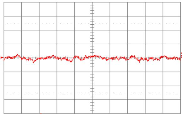
Figure 1.2V.22. Input reflected ripple current,  $i_s$  (10 mA/div.), measured through  $10 \mu\text{H}$  at the source at full rated load current and  $V_{in} = 48 \text{ V}$ . Refer to Fig. 1.2V.20 for test setup. Time scale:  $1 \mu\text{s}/\text{div}$ .
