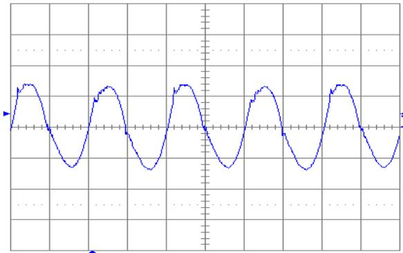
Figure 3.3V.19. Output voltage ripple (20 mV/div.) at full rated load current into a resistive load with  $C_o = 10 \mu\text{F}$  tantalum +  $1 \mu\text{F}$  ceramic and  $V_{in} = 48 \text{ V}$ . Time scale:  $1 \mu\text{s}/\text{div}$ .
