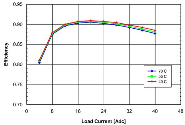
Figure 2.5V.12. Efficiency vs. load current and ambient temperature for QME48T40025 converter mounted horizontally with  $V_{in} = 48\text{ V}$  and air flowing from pin 1 to pin 3 at a rate of 200 LFM (1.0 m/s).
