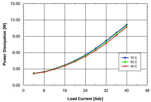
Figure 1.2V.14. Power dissipation vs. load current and ambient temperature for QME48T40012 converter mounted horizontally with  $V_{in} = 48\text{ V}$  and air flowing from pin 1 to pin 3 at a rate of 200 LFM (1.0 m/s).
