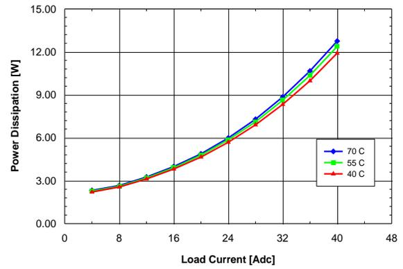
Figure 1.8V.14. Power dissipation vs. load current and ambient temperature for QME48T40018 converter mounted horizontally with  $V_{in} = 48\text{ V}$  and air flowing from pin 1 to pin 3 at a rate of 200 LFM (1.0 m/s).
