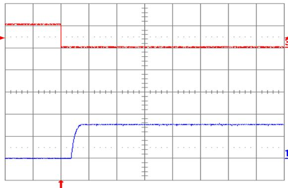
Figure 1.5V.15. Turn-on transient at full rated load current (resistive) with no output capacitor at  $V_{in} = 48\text{ V}$ , triggered via ON/OFF pin. Top trace: ON/OFF signal (5 V/div.). Bottom trace: output voltage (1 V/div.). Time scale: 2 ms/div.
