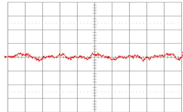
Figure 1.5V.22. Input reflected ripple current,  $i_s$  (10 mA/div.), measured through  $10 \mu\text{H}$  at the source at full rated load current and  $V_{in} = 48 \text{ V}$ . Refer to Fig. 1.5V.20 for test setup. Time scale:  $1 \mu\text{s}/\text{div}$ .
