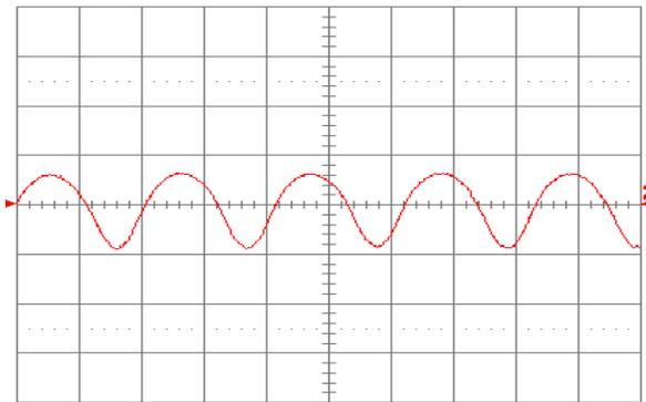
Figure 1.5V.21. Input reflected ripple current,  $i_c$  (100 mA/div.), measured at input terminals at full rated load current and  $V_{in} = 48 \text{ V}$ . Refer to Fig. 1.5V.20 for test setup. Time scale:  $1 \mu\text{s}/\text{div}$ .
