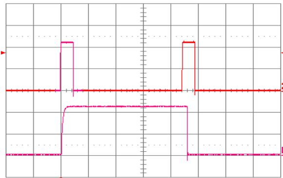
Figure 1.2V.24. Load current (top trace, 20 A/div., 50 ms/div.) into a  $10 \text{ m}\Omega$  short circuit during restart, at  $V_{in} = 48 \text{ V}$ . Bottom trace (20 A/div., 5 ms/div.) is an expansion of the on-time portion of the top trace.
