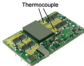
Figure 8. Location of the thermocouple for thermal testing.
