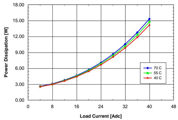
Figure 3.3V.14. Power dissipation vs. load current and ambient temperature for QME48T40033 converter mounted horizontally with  $V_{in} = 48\text{ V}$  and air flowing from pin 1 to pin 3 at a rate of 200 LFM (1.0 m/s).
