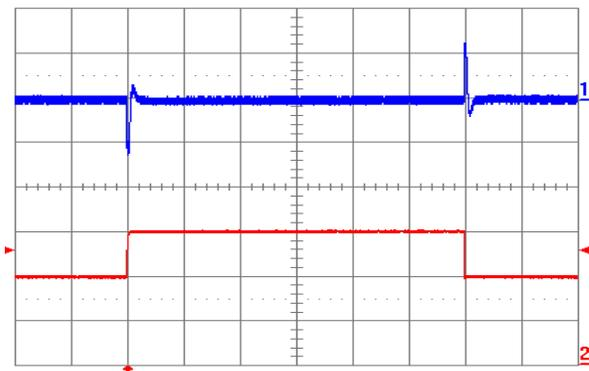
Figure 1.8V.18. Output voltage response to load current step-change (20 A – 30 A – 20 A) at  $V_{in} = 48\text{ V}$ . Top trace: output voltage (100 mV/div.). Bottom trace: load current (10 A/div.). Current slew rate: 5 A/ $\mu\text{s}$ .  $C_o = 470\ \mu\text{F}$  POS + 1  $\mu\text{F}$  ceramic. Time scale: 0.2 ms/div.
