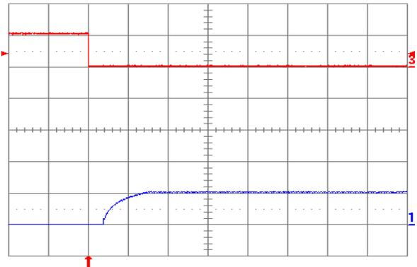
Figure 1.0V.16. Turn-on transient at full rated load current (resistive) plus 10,000  $\mu\text{F}$  at  $V_{in} = 48\text{ V}$ , triggered via ON/OFF pin. Top trace: ON/OFF signal (5 V/div.). Bottom trace: output voltage (1 V/div.). Time scale: 2 ms/div.
