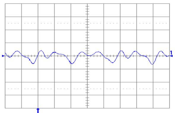
Figure 1.0V.18. Output voltage response to load current step-change (20 A – 30 A – 20 A) at  $V_{in} = 48\text{ V}$ . Top trace: output voltage (100 mV/div.). Bottom trace: load current (10 A/div.). Current slew rate: 5 A/ $\mu\text{s}$ .  $C_o = 470\text{ }\mu\text{F POS} + 1\text{ }\mu\text{F}$  ceramic. Time scale: 0.2 ms/div.
