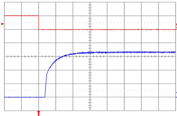
Figure 3.3V.15. Turn-on transient at full rated load current (resistive) with no output capacitor at  $V_{in} = 48\text{ V}$ , triggered via ON/OFF pin. Top trace: ON/OFF signal (5 V/div.). Bottom trace: output voltage (1 V/div.). Time scale: 2 ms/div.
