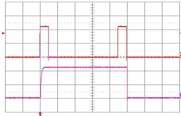
Figure 1.0V.24. Load current (top trace, 20 A/div., 50 ms/div.) into a  $10 \text{ m}\Omega$  short circuit during restart, at  $V_{in} = 48 \text{ V}$ . Bottom trace (20 A/div., 5 ms/div.) is an expansion of the on-time portion of the top trace.
