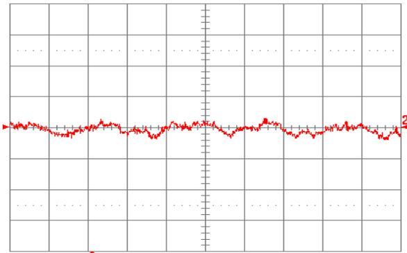
Figure 3.3V.22. Input ripple current,  $i_s$  (10 mA/div.), measured through  $10 \mu\text{H}$  at the source at full rated load current and  $V_{in} = 48 \text{ V}$ . Refer to Fig. 3.3V.20 for test setup. Time scale:  $1 \mu\text{s}/\text{div}$ .
