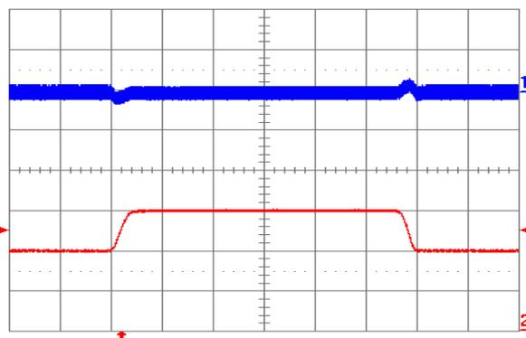
Figure 1.5V.17. Output voltage response to load current step-change (20 A – 30 A – 20 A) at  $V_{in} = 48\text{ V}$ . Top trace: output voltage (100 mV/div.). Bottom trace: load current (10 A/div.). Current slew rate: 0.1 A/ $\mu\text{s}$ .  $C_o = 1\ \mu\text{F}$  ceramic. Time scale: 0.2 ms/div.
