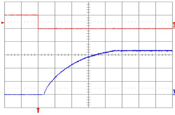
Figure 3.3V.16. Turn-on transient at full rated load current (resistive) plus 10,000  $\mu\text{F}$  at  $V_{in} = 48\text{ V}$ , triggered via ON/OFF pin. Top trace: ON/OFF signal (5 V/div.). Bottom trace: output voltage (1 V/div.). Time scale: 2 ms/div.
