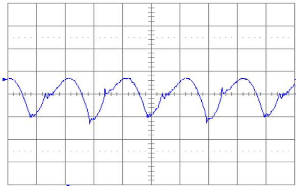
Figure 1.2V.19. Output voltage ripple (20 mV/div.) at full rated load current into a resistive load with  $C_o = 10 \mu\text{F}$  tantalum +  $1 \mu\text{F}$  ceramic and  $V_{in} = 48 \text{ V}$ . Time scale:  $1 \mu\text{s}/\text{div}$ .
