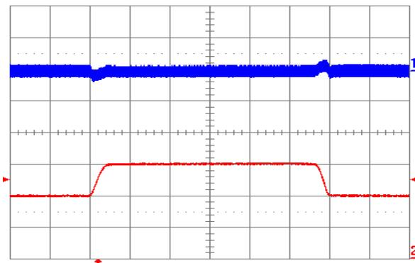
Figure 1.8V.17. Output voltage response to load current step-change (20 A – 30 A – 20 A) at  $V_{in} = 48\text{ V}$ . Top trace: output voltage (100 mV/div.). Bottom trace: load current (10 A/div.). Current slew rate: 0.1 A/ $\mu\text{s}$ .  $C_o = 1\ \mu\text{F}$  ceramic. Time scale: 0.2 ms/div.
