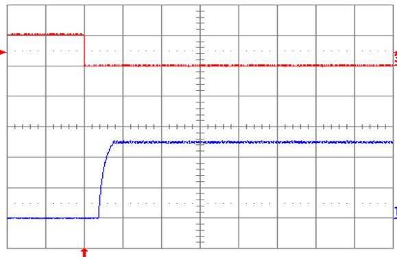
Figure 2.5V.15. Turn-on transient at full rated load current (resistive) with no output capacitor at  $V_{in} = 48\text{ V}$ , triggered via ON/OFF pin. Top trace: ON/OFF signal (5 V/div.). Bottom trace: output voltage (1 V/div.). Time scale: 2 ms/div.
