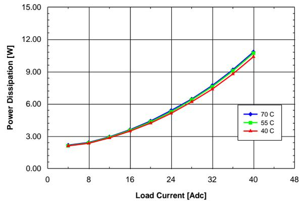
Figure 1.0V.14. Power dissipation vs. load current and ambient temperature for QME48T40010 converter mounted horizontally with  $V_{in} = 48\text{ V}$  and air flowing from pin 1 to pin 3 at a rate of 200 LFM (1.0 m/s).
