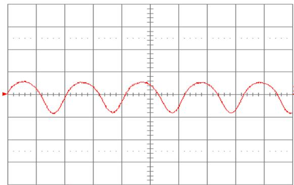
Figure 1.2V.21. Input reflected ripple current,  $i_c$  (100 mA/div.), measured at input terminals at full rated load current and  $V_{in} = 48 \text{ V}$ . Refer to Fig. 1.2V.20 for test setup. Time scale:  $1 \mu\text{s}/\text{div}$ .
