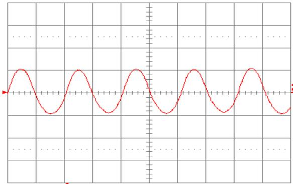
Figure 3.3V.21. Input reflected ripple current,  $i_c$  (100 mA/div.), measured at input terminals at full rated load current and  $V_{in} = 48 \text{ V}$ . Refer to Fig. 3.3V.20 for test setup. Time scale:  $1 \mu\text{s}/\text{div}$ .
