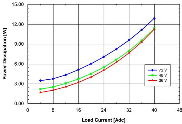
Figure 1.8V.13. Power dissipation vs. load current and input voltage for QME48T40018 converter mounted horizontally with air flowing from pin 1 to pin 3 at a rate of 300 LFM (1.5 m/s) and  $T_a = 25^\circ\text{C}$ .
