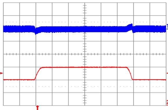
Figure 2.5V.17. Output voltage response to load current step-change (20 A – 30 A – 20 A) at  $V_{in} = 48\text{ V}$ . Top trace: output voltage (100 mV/div.). Bottom trace: load current (10 A/div.). Current slew rate: 0.1 A/ $\mu\text{s}$ .  $C_o = 1\ \mu\text{F}$  ceramic. Time scale: 0.2 ms/div.
