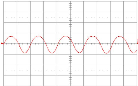
Figure 1.8V.21. Input reflected ripple current,  $i_c$  (100 mA/div.), measured at input terminals at full rated load current and  $V_{in} = 48 \text{ V}$ . Refer to Fig. 1.8V.20 for test setup. Time scale:  $1 \mu\text{s}/\text{div}$ .
