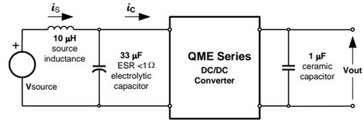
Figure 3.3V.20. Test setup for measuring input reflected ripple currents,  $i_c$  and  $i_s$ .
