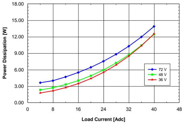
Figure 2.5V.13. Power dissipation vs. load current and input voltage for QME48T40025 converter mounted horizontally with air flowing from pin 1 to pin 3 at a rate of 300 LFM (1.5 m/s) and  $T_a = 25^\circ\text{C}$ .
