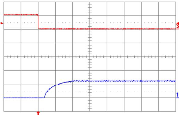
Figure 1.2V.16. Turn-on transient at full rated load current (resistive) plus 10,000  $\mu\text{F}$  at  $V_{in} = 48\text{ V}$ , triggered via ON/OFF pin. Top trace: ON/OFF signal (5 V/div.). Bottom trace: output voltage (1 V/div.). Time scale: 2 ms/div.
