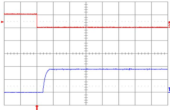
Figure 1.8V.15. Turn-on transient at full rated load current (resistive) with no output capacitor at  $V_{in} = 48\text{ V}$ , triggered via ON/OFF pin. Top trace: ON/OFF signal (5 V/div.). Bottom trace: output voltage (1 V/div.). Time scale: 2 ms/div.
