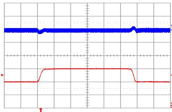
Figure 1.2V.17. Output voltage response to load current step-change (20 A – 30 A – 20 A) at  $V_{in} = 48\text{ V}$ . Top trace: output voltage (100 mV/div.). Bottom trace: load current (10 A/div.). Current slew rate: 0.1 A/ $\mu\text{s}$ .  $C_o = 1\ \mu\text{F}$  ceramic. Time scale: 0.2 ms/div.
