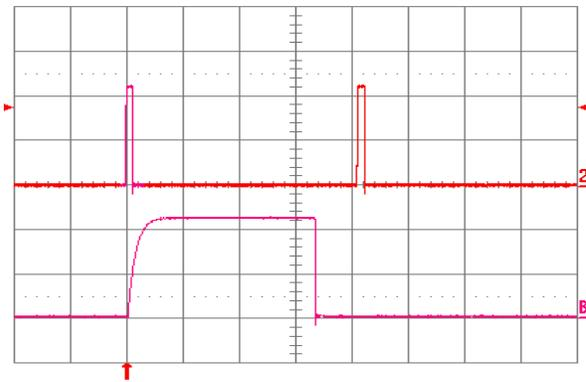
Figure 3.3V.24. Load current (top trace, 20 A/div., 50 ms/div.) into a  $10 \text{ m}\Omega$  short circuit during restart, at  $V_{in} = 48 \text{ V}$ . Bottom trace (20 A/div., 2 ms/div.) is an expansion of the on-time portion of the top trace.
