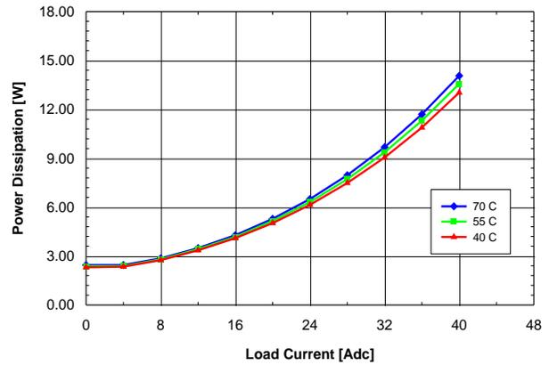
Figure 2.5V.14. Power dissipation vs. load current and ambient temperature for QME48T40025 converter mounted horizontally with  $V_{in} = 48\text{ V}$  and air flowing from pin 1 to pin 3 at a rate of 200 LFM (1.0 m/s).
