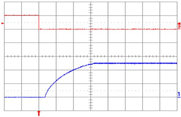
Figure 2.5V.16. Turn-on transient at full rated load current (resistive) plus 10,000  $\mu\text{F}$  at  $V_{in} = 48\text{ V}$ , triggered via ON/OFF pin. Top trace: ON/OFF signal (5 V/div.). Bottom trace: output voltage (1 V/div.). Time scale: 2 ms/div.
