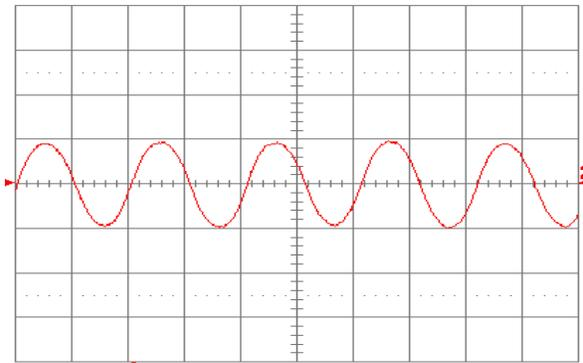
Figure 2.5V.21. Input reflected ripple current,  $i_c$  (100 mA/div.), measured at input terminals at full rated load current and  $V_{in} = 48 \text{ V}$ . Refer to Fig. 2.5V.20 for test setup. Time scale: 1  $\mu\text{s}/\text{div}$ .
