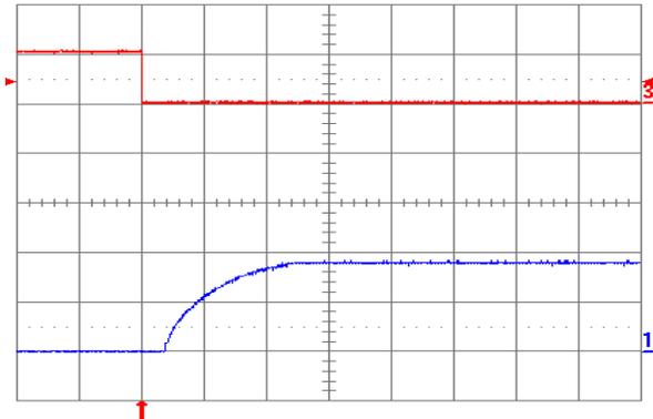
Figure 1.8V.16. Turn-on transient at full rated load current (resistive) plus 10,000  $\mu\text{F}$  at  $V_{in} = 48\text{ V}$ , triggered via ON/OFF pin. Top trace: ON/OFF signal (5 V/div.). Bottom trace: output voltage (1 V/div.). Time scale: 2 ms/div.
