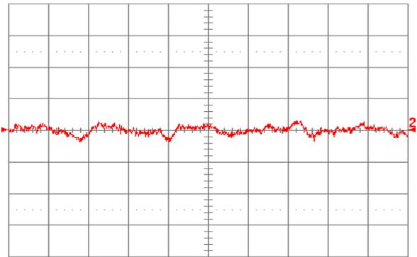
Figure 1.8V.22. Input reflected ripple current,  $i_s$  (10 mA/div.), measured through  $10 \mu\text{H}$  at the source at full rated load current and  $V_{in} = 48 \text{ V}$ . Refer to Fig. 1.8V.20 for test setup. Time scale:  $1 \mu\text{s}/\text{div}$ .
