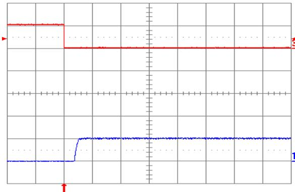
Figure 1.0V.15. Turn-on transient at full rated load current (resistive) with no output capacitor at  $V_{in} = 48\text{ V}$ , triggered via ON/OFF pin. Top trace: ON/OFF signal (5 V/div.). Bottom trace: output voltage (1 V/div.). Time scale: 2 ms/div
