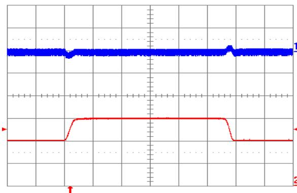
Figure 1.0V.17. Output voltage response to load current step-change (20 A – 30 A – 20 A) at  $V_{in} = 48\text{ V}$ . Top trace: output voltage (100 mV/div.). Bottom trace: load current (10 A/div.). Current slew rate: 0.1 A/ $\mu\text{s}$ .  $C_o = 1\text{ }\mu\text{F}$  ceramic. Time scale: 0.2 ms/div.
