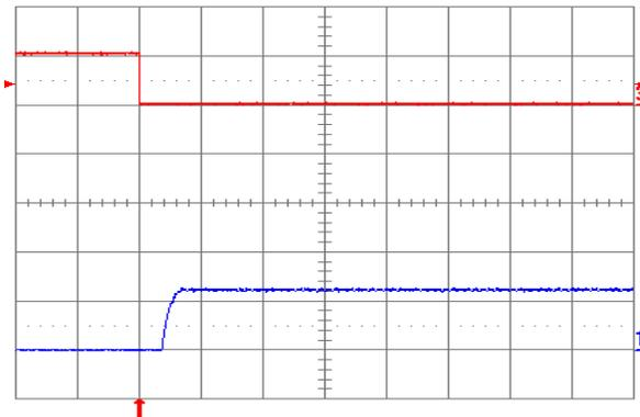
Figure 1.2V.15. Turn-on transient at full rated load current (resistive) with no output capacitor at  $V_{in} = 48\text{ V}$ , triggered via ON/OFF pin. Top trace: ON/OFF signal (5 V/div.). Bottom trace: output voltage (1 V/div.). Time scale: 2 ms/div.
