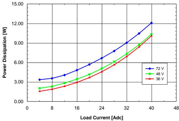
Figure 1.2V.13. Power dissipation vs. load current and input voltage for QME48T40012 converter mounted horizontally with air flowing from pin 1 to pin 3 at a rate of 300 LFM (1.5 m/s) and  $T_a = 25^\circ\text{C}$ .
