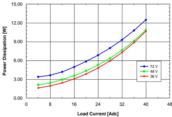
Figure 1.5V.13. Power dissipation vs. load current and input voltage for QME48T40015 converter mounted horizontally with air flowing from pin 1 to pin 3 at a rate of 300 LFM (1.5 m/s) and  $T_a = 25^\circ\text{C}$ .
