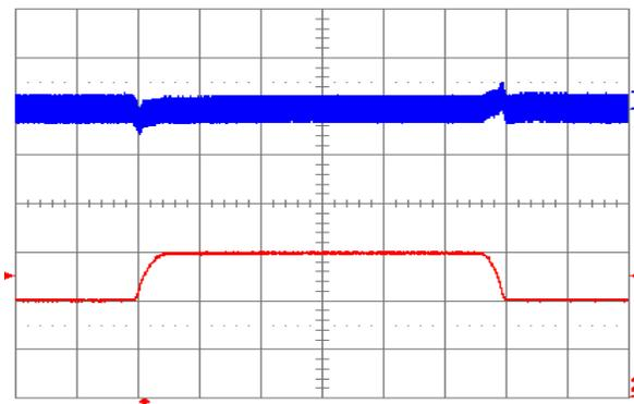
Figure 3.3V.17. Output voltage response to load current step-change (20 A – 30 A – 20 A) at  $V_{in} = 48\text{ V}$ . Top trace: output voltage (100 mV/div.). Bottom trace: load current (10 A/div.). Current slew rate: 0.1 A/ $\mu\text{s}$ .  $C_o = 1\ \mu\text{F}$  ceramic. Time scale: 0.2 ms/div.
