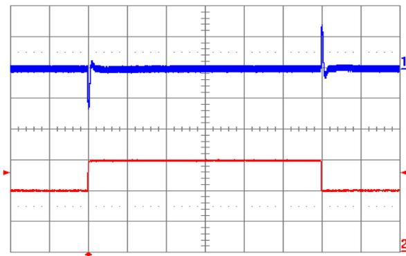
Figure 3.3V.18. Output voltage response to load current step-change (20 A – 30 A – 20 A) at  $V_{in} = 48\text{ V}$ . Top trace: output voltage (100 mV/div.). Bottom trace: load current (10 A/div.). Current slew rate: 5 A/ $\mu\text{s}$ .  $C_o = 470\ \mu\text{F}$  POS + 1  $\mu\text{F}$  ceramic. Time scale: 0.2 ms/div.
