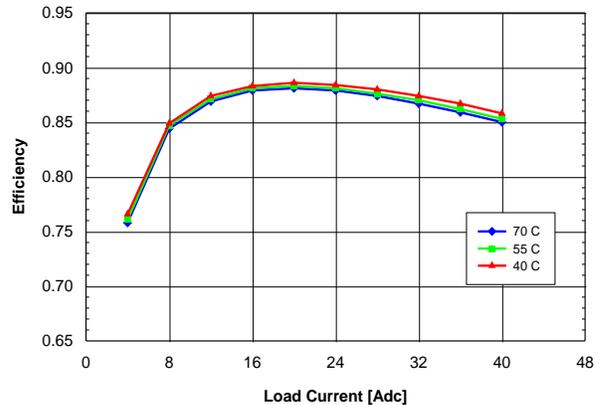
Figure 1.8V.12. Efficiency vs. load current and ambient temperature for QME48T40018 converter mounted horizontally with  $V_{in} = 48\text{ V}$  and air flowing from pin 1 to pin 3 at a rate of 200 LFM (1.0 m/s).
