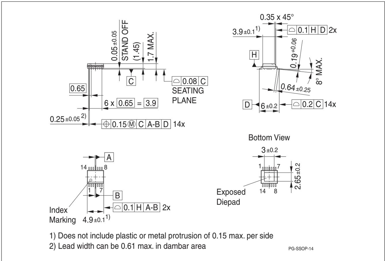
Figure 13 PG-SSOP-14
