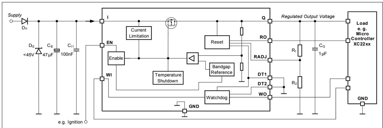
Figure 12 Application Diagram
