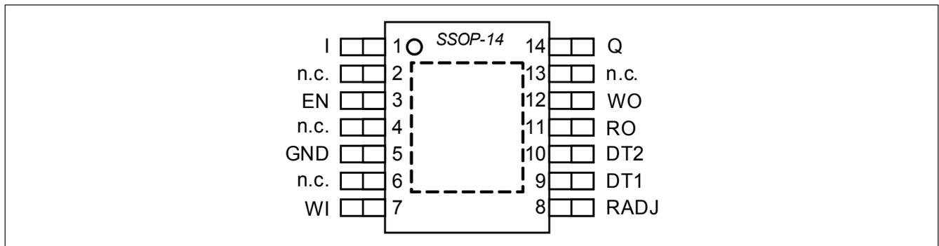
Figure 3 Pin Configuration
