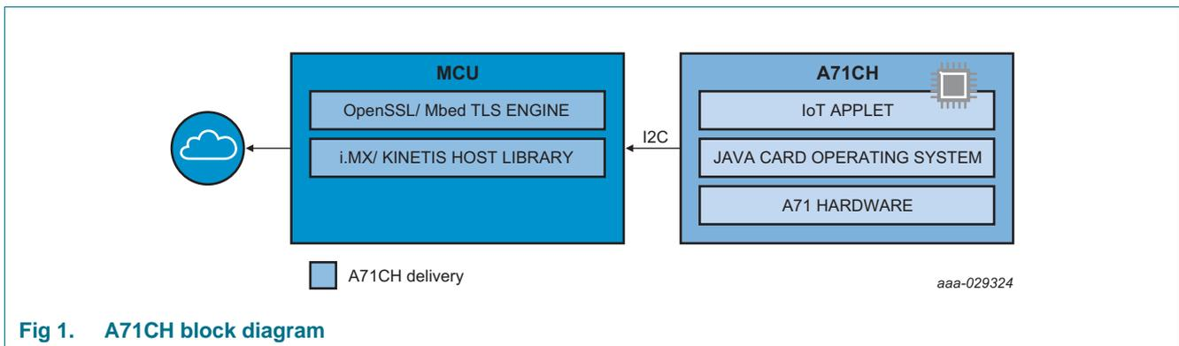
Fig 1. A71CH block diagram
