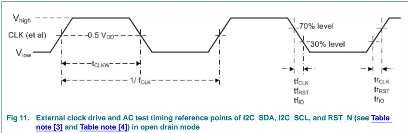
**Fig 11. External clock drive and AC test timing reference points of I2C\_SDA, I2C\_SCL, and RST\_N (see [Table note \[3\]](#) and [Table note \[4\]](#)) in open drain mode**
