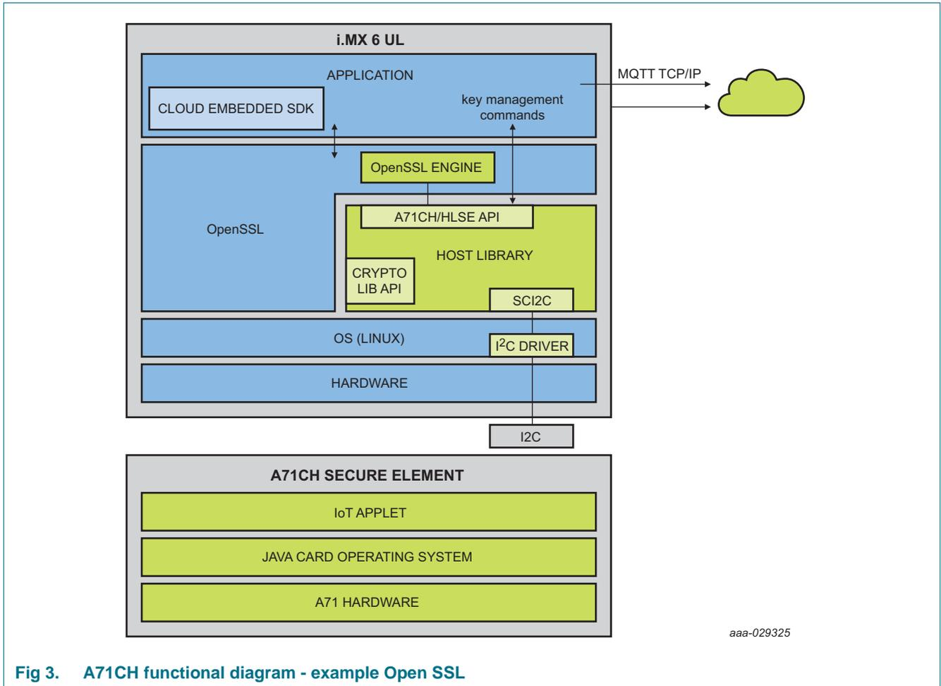
Fig 3. A71CH functional diagram - example Open SSL
