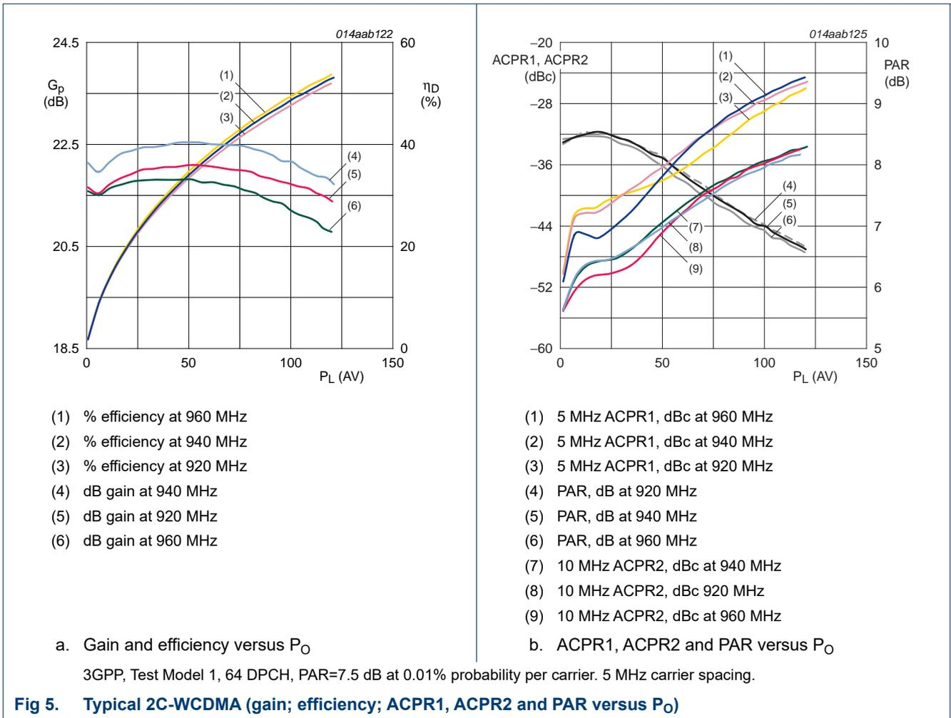
Fig 5. Typical 2C-WCDMA (gain; efficiency; ACPR1, ACPR2 and PAR versus  $P_O$ )
