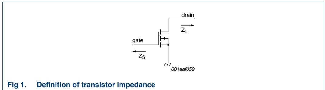
**Fig 1. Definition of transistor impedance**
