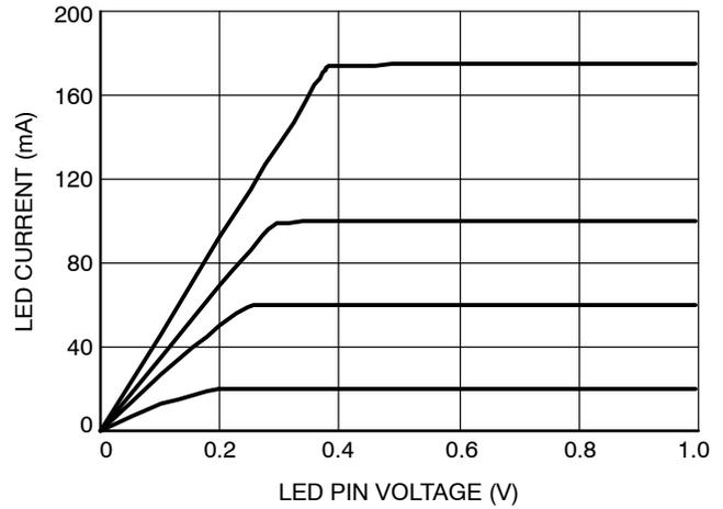
Figure 6. LED Current vs. LED Pin Voltage
