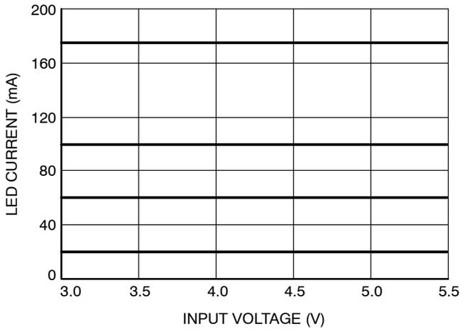
Figure 7. LED Current Change vs. Input Voltage
