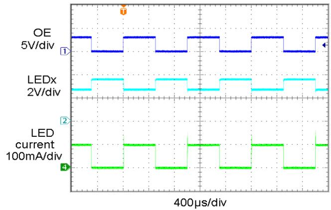
Figure 12. OE Transient Response at 1 kHz
