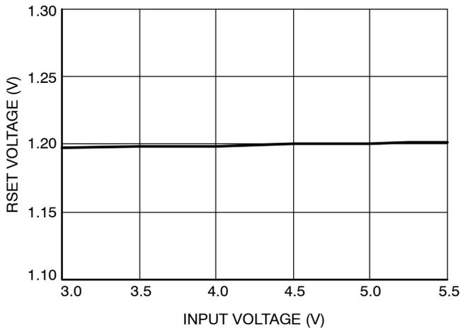
Figure 9. RSET Pin Voltage vs. Input Voltage
