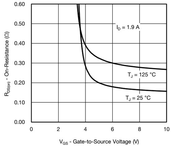
R<sub>DS(on)</sub> vs. V<sub>GS</sub> vs. Temperature
