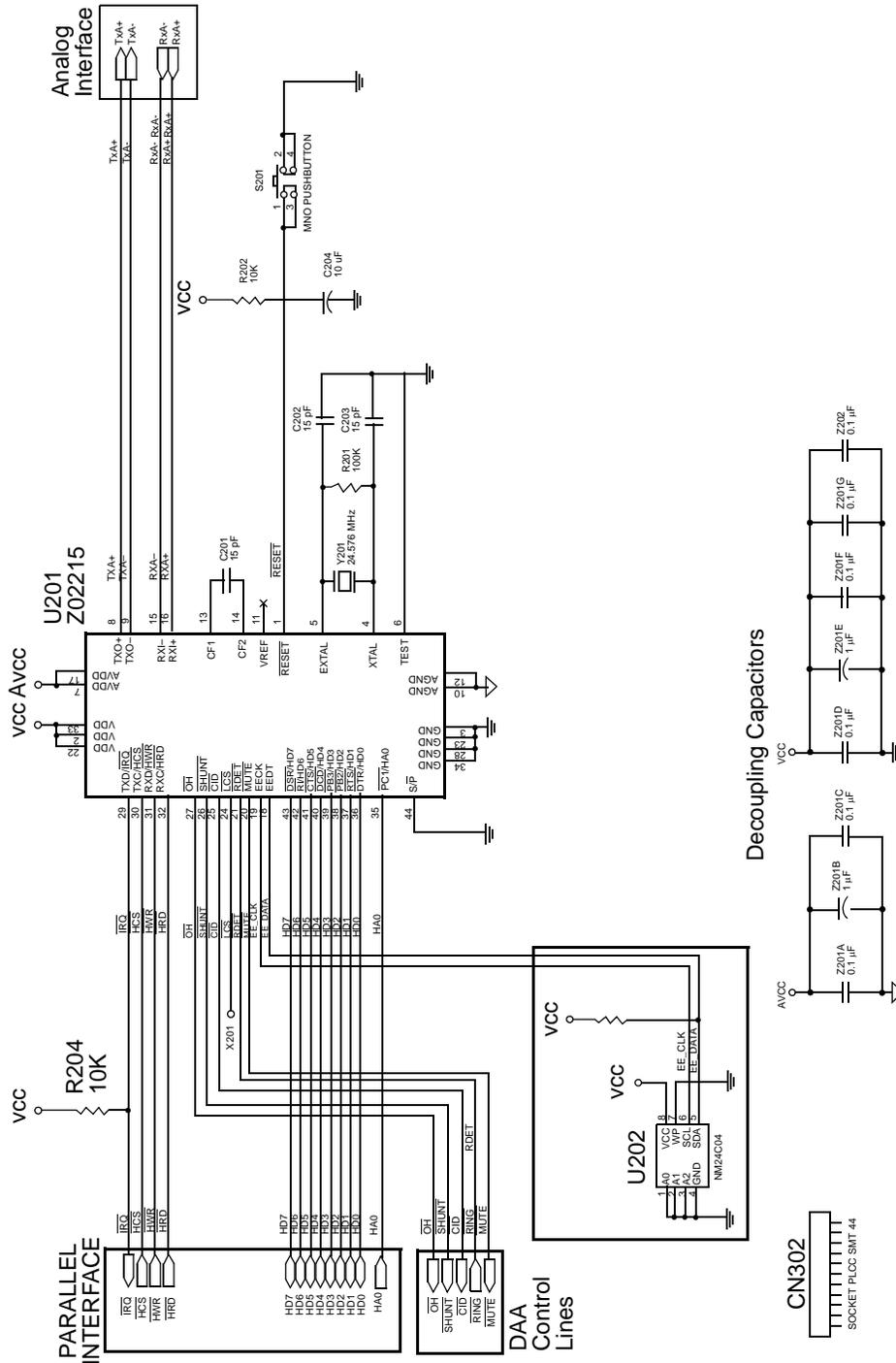
Figure 9. Typical Modem Employing the Z02215 (Parallel Mode)
