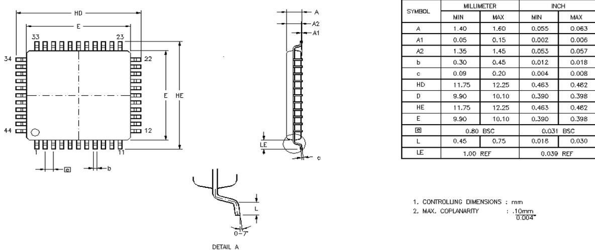
Figure 14. 44-Lead LQFP Package Diagram
