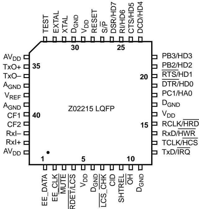
Figure 3. Z02215 44-Lead LQFP Pin Identification
