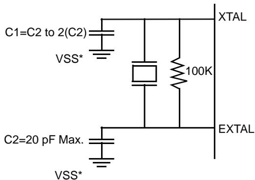
$C_1, C_2$  – The C values are dependent on the load capacitance of the chosen crystal. Refer to the Application Note titled *Crystal Oscillator for Embedded Modems* at:
