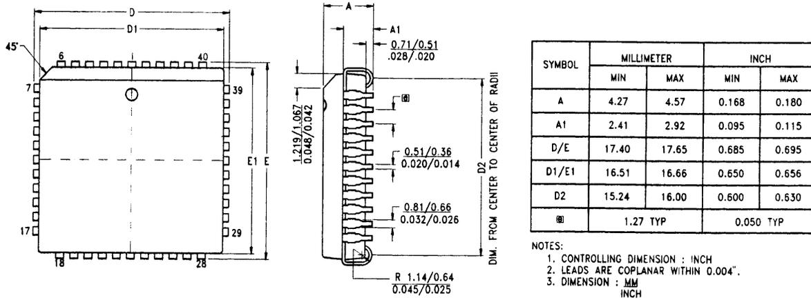
Figure 13. 44-Lead PLCC Package Diagram (for Prototype Only)
