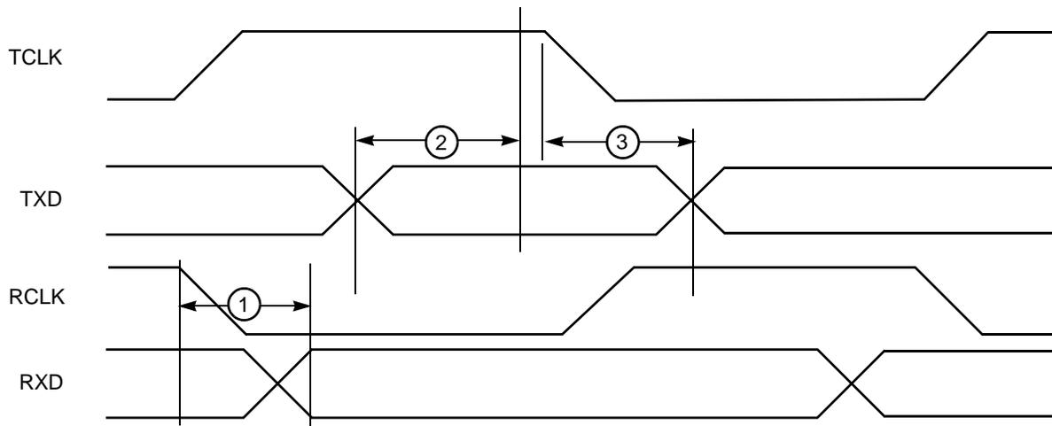
**Figure 11. Serial Port Timing Diagram**
