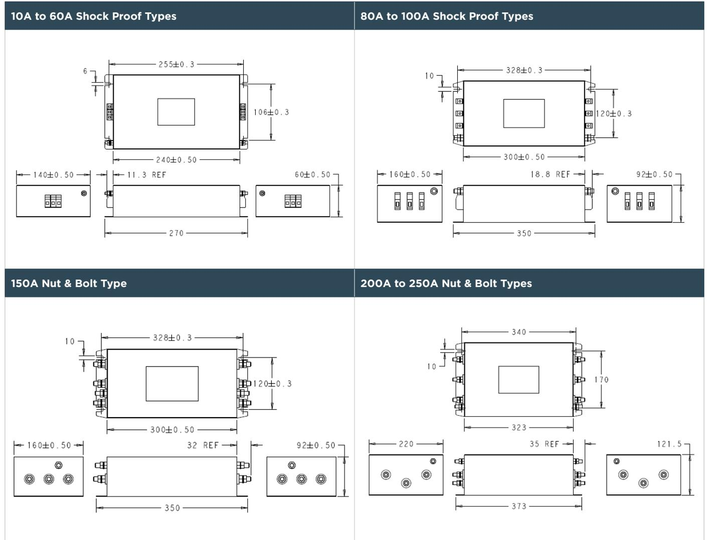
All dimensions in mm; Tolerances according: ISO2768-m
