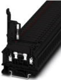
Fuse modular terminal block, Number of positions: 1, Connection method: Screw connection, Cross section: 0.2 mm<sup>2</sup>- 6 mm<sup>2</sup>, AWG: 24 - 10, Nominal current: 6.3 A, Nominal voltage: 500 V, Width: 8.2 mm, Fuse type: G / 5 x 20, Fuse type: Glass, Mounting type: NS 35/7,5, NS 35/15, NS 32, Color: black
