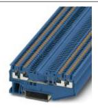
Disconnect terminal block, Connection type: Push-in connection, Cross section: 0.14 mm² - 1.5 mm², AWG: 26 - 16, Nominal current: 10 A, Nominal voltage: 400 V, Length: 76.9 mm, Width: 3.5 mm, Color: blue, Assembly: NS 35/7,5, NS 35/15
