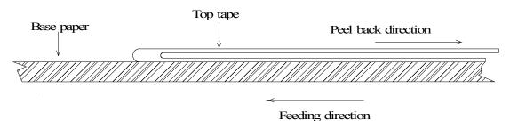
4.2 Base tape should not adhere to top tape when top tape is peeled back, and peel back direction is as follows.
