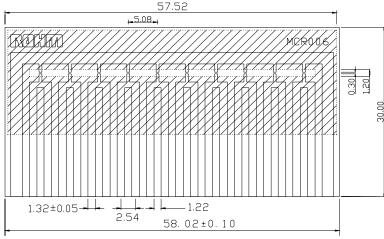
NOTE) \*1 The shaded area shows the solder resist treatment.
