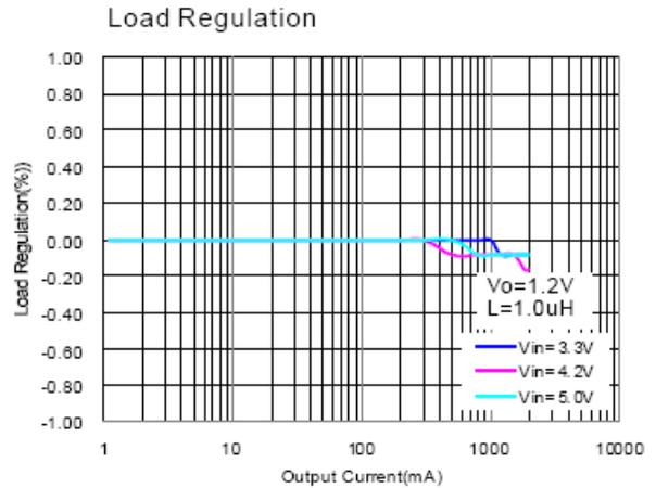
**Typical Performance Characteristics** (cont.) (@T<sub>A</sub> = +25°C, C<sub>IN</sub> = 22\*2μF, C<sub>O</sub> = 22μF, unless otherwise specified.)
