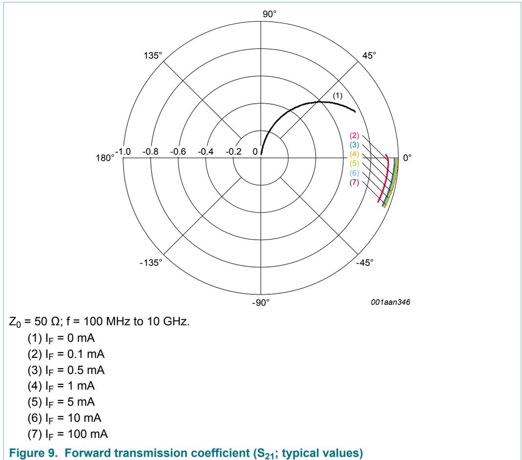
**7.2.2 Diode in parallel configuration**
