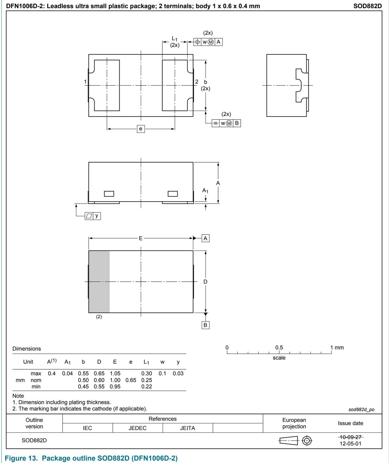
**Figure 13. Package outline SOD882D (DFN1006D-2)**
