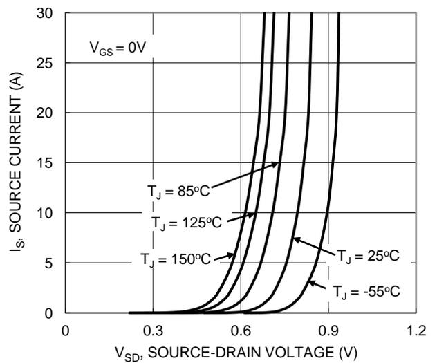
Figure 18. Q2 Diode Forward Voltage vs. Current
