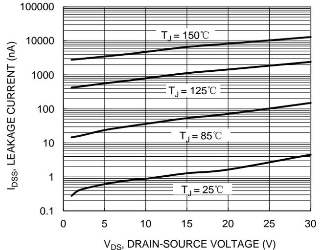
Figure 20. Q2 Typical Drain-Source Leakage Current vs. Voltage
