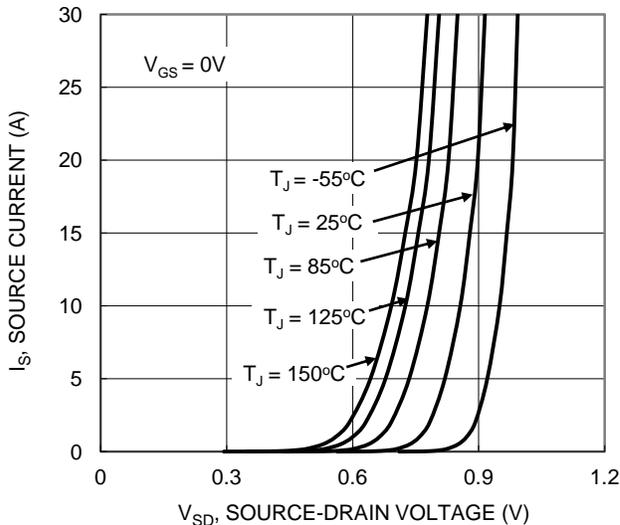
Figure 17. Q1 Diode Forward Voltage vs. Current
