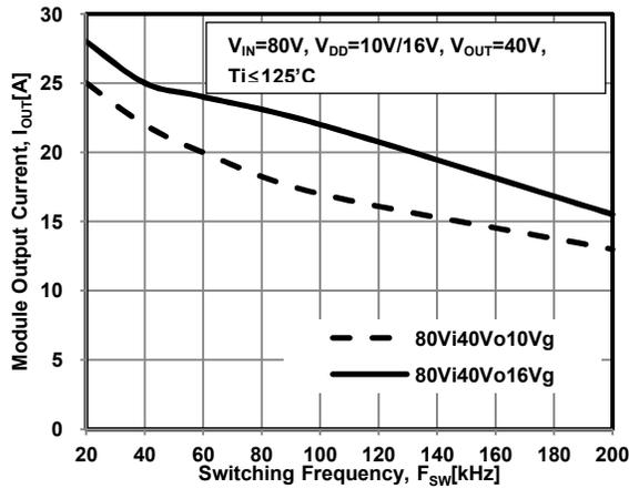
Figure 33. Static SOA, V<sub>IN</sub>=80V
