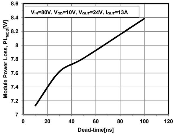
Figure 35. Module Power Loss vs. T<sub>DEAD</sub>
