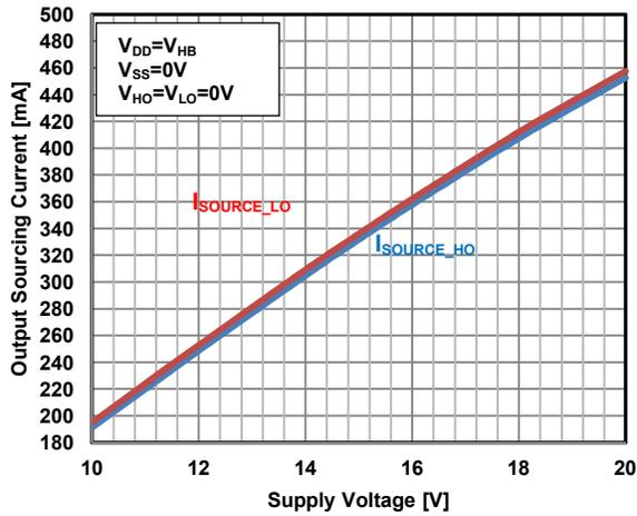
Figure 21. Output Sourcing Current vs. Supply Voltage (V<sub>DD</sub>)
