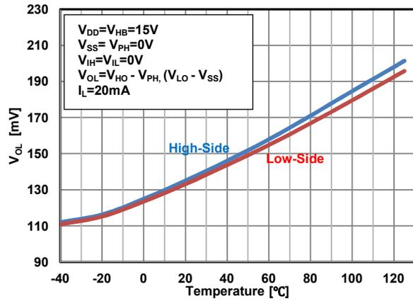
Figure 28. Low-Level Output Voltage Deviation from the V<sub>PH</sub>(V<sub>SS</sub>) vs. Temp.
