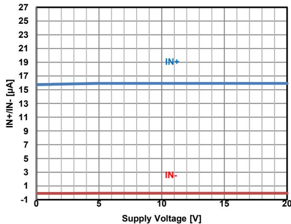
Figure 31. I<sub>N+</sub> I<sub>N-</sub> vs. Supply Voltage(V<sub>DD</sub>)
