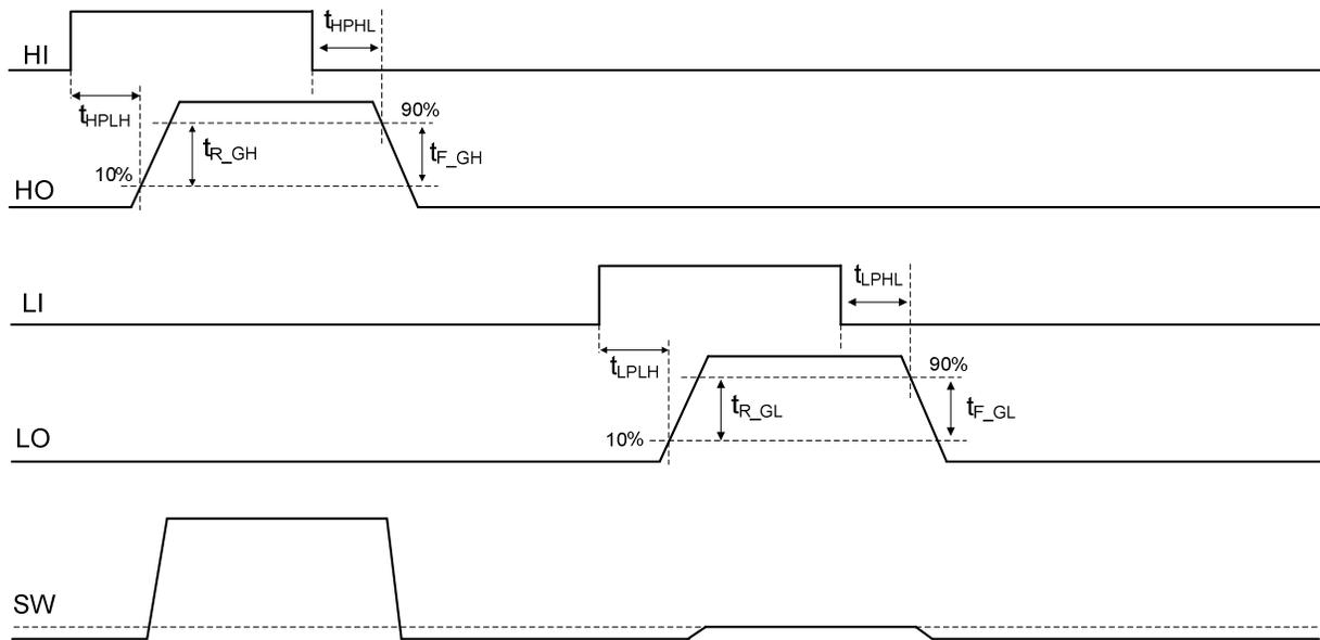
Figure 64. PWM Timing Diagram (LI / HI signals)
