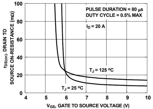
Figure 53. On-Resistance vs. Gate to Source Voltage
