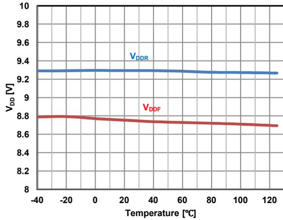
Figure 29. V<sub>DD</sub> UVLO Threshold Voltage vs. Temp.
