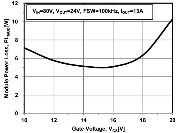
Figure 36. Module Power Loss vs. V<sub>GS</sub>
