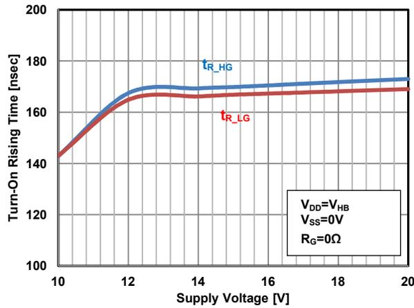
Figure 17. Turn-On Rising Time vs. Supply Voltage (V<sub>DD</sub>)
