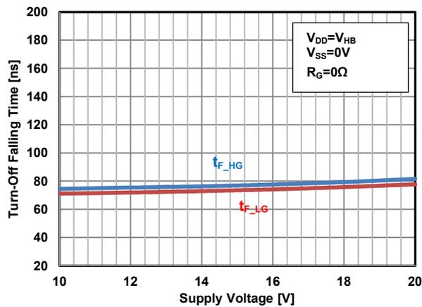
Figure 19. Turn-Off Falling Time vs. Supply Voltage (V<sub>DD</sub>)
