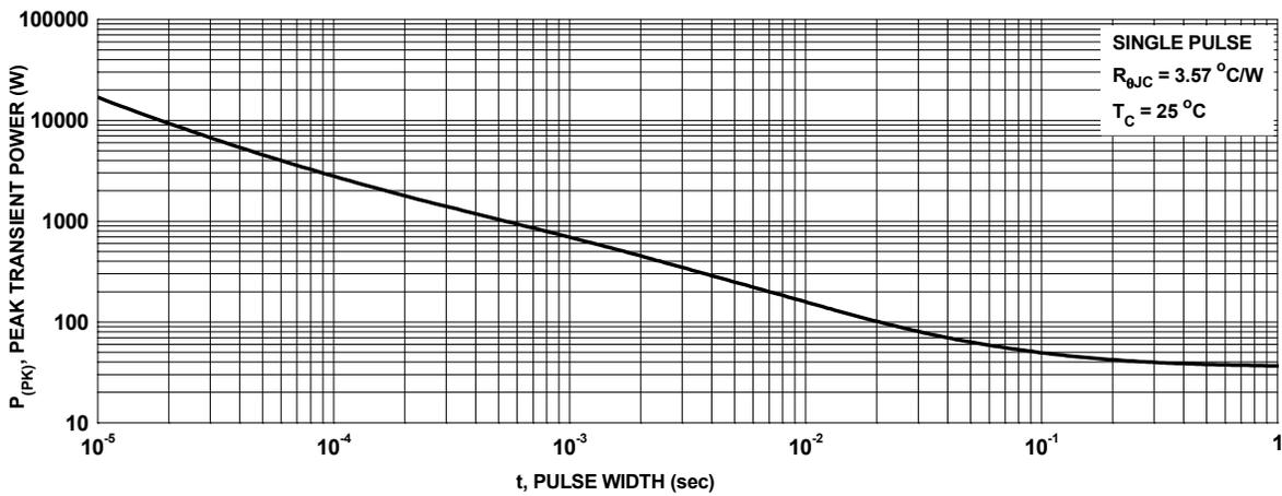
Figure 60. Single Pulse Maximum Power Dissipation
