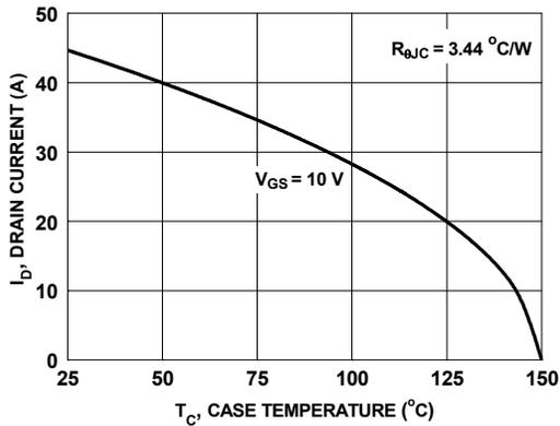
Figure 46. Maximum Continuous Drain Current vs. Case Temperature
