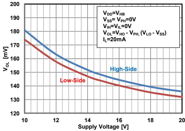
Figure 27. Low-Level Output Voltage Deviation from the V<sub>PH</sub>(V<sub>SS</sub>) vs. Supply Voltage(V<sub>DD</sub>)
