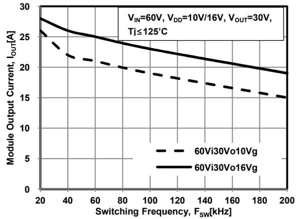
Figure 34. Static SOA, V<sub>IN</sub>=60V
