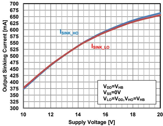
Figure 23. Output Sinking Current vs. Supply Voltage (V<sub>DD</sub>)
