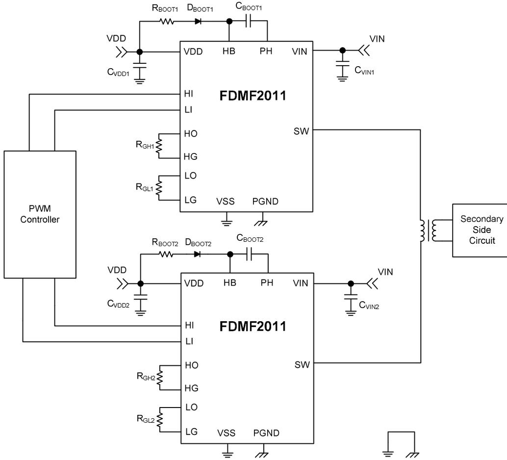
Figure 8. Full-Bridge Converter
