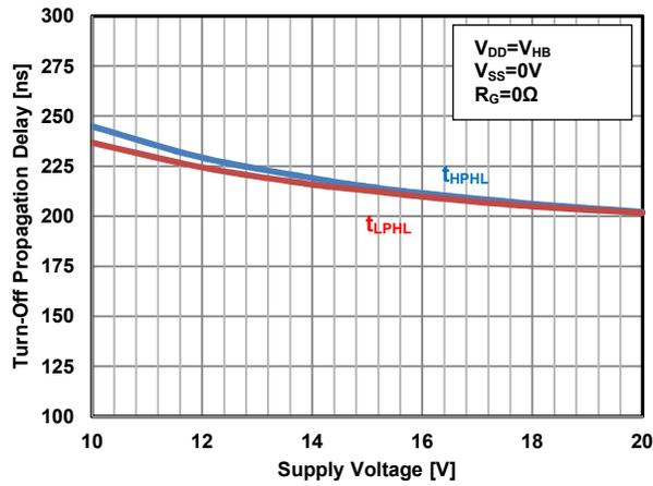
Figure 15. Turn-Off Propagation Delay vs. Supply Voltage (V<sub>DD</sub>)
