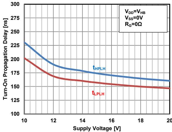
Figure 13. Turn-On Propagation Delay vs. Supply Voltage(V<sub>DD</sub>)
