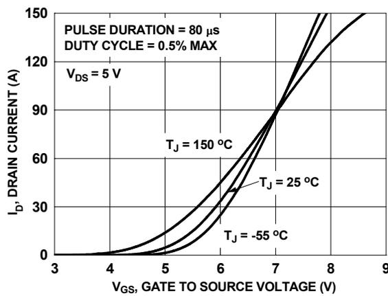
Figure 54. Transfer Characteristics
