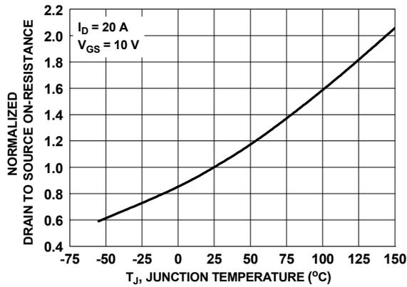
Figure 52. Normalized On Resistance vs. Junction Temperature
