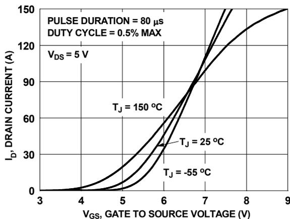
Figure 42. Transfer Characteristics
