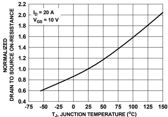
Figure 40. Normalized On Resistance vs. Junction Temperature
