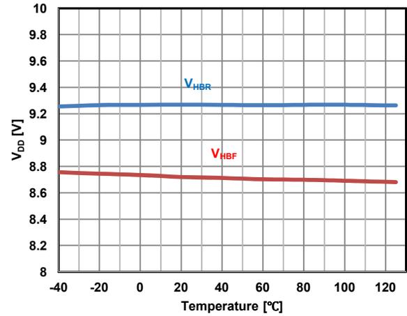
Figure 30. V<sub>HB</sub> UVLO Threshold Voltage vs. Temp.
