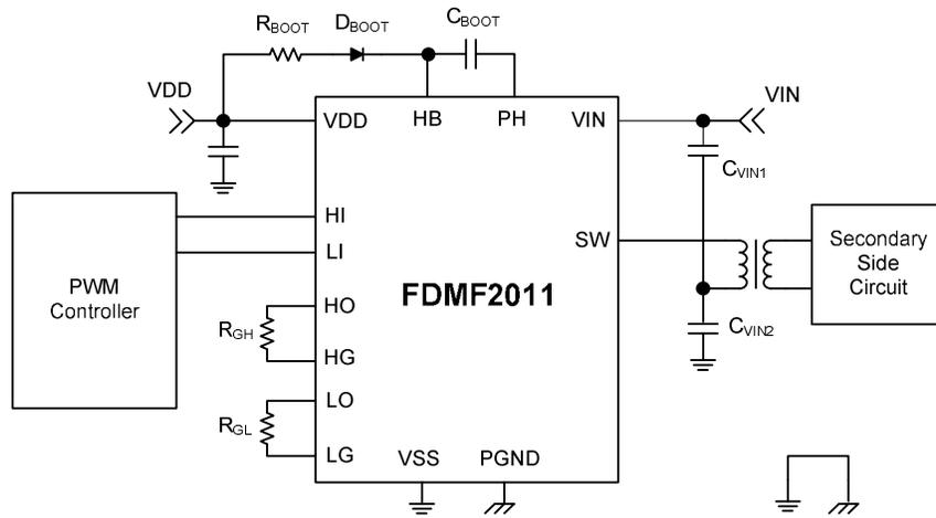
**Figure 7. Half-Bridge Converter**
