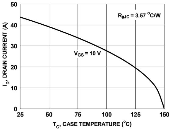
Figure 58. Maximum Continuous Drain Current vs. Case Temperature
