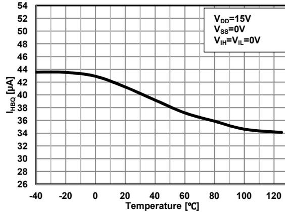
Figure 12. I<sub>HBQ</sub> vs. Temp.
