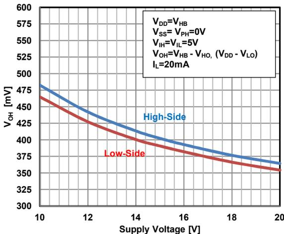
Figure 25. High-Level Output Voltage Deviation from the V<sub>BH</sub> (V<sub>DD</sub>) vs. Supply Voltage (V<sub>DD</sub>)
