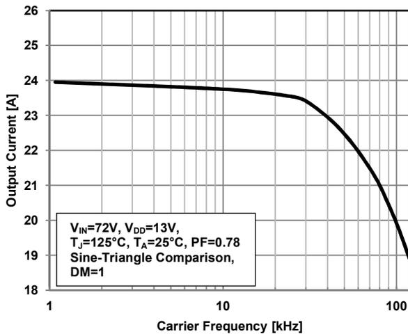
Figure 37. Output Current Vs. Carrier or Modulation Frequency
