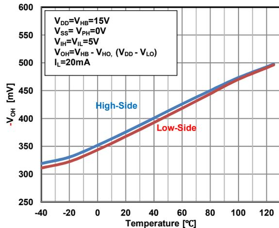
Figure 26. High-Level Output Voltage Deviation from the V<sub>BH</sub> (V<sub>DD</sub>) vs. Temp.
