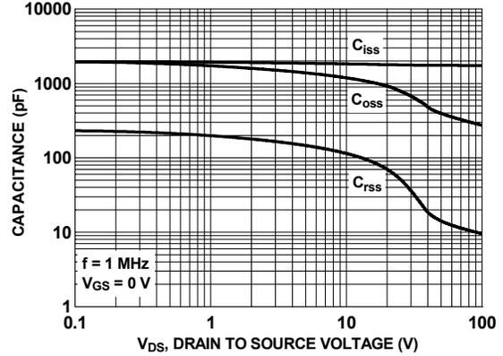
Figure 45. Capacitance vs. Drain to Source Voltage
