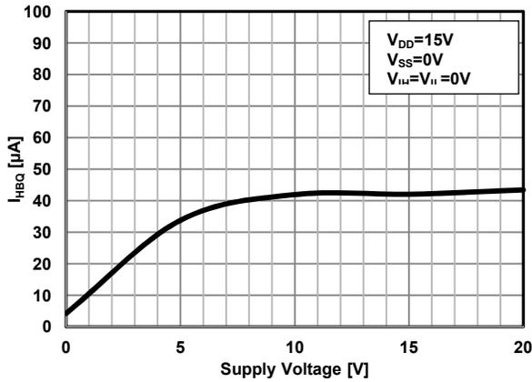
Figure 11. I<sub>HBQ</sub> vs. Supply Voltage(V<sub>DD</sub>)
