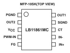
V<sub>CC</sub>: Common power supply for motor and control systems
