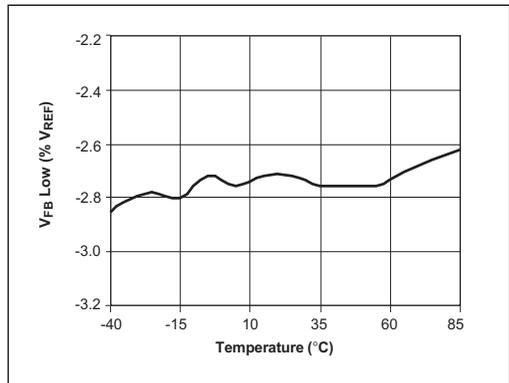
Figure 13.  $V_{FB}$  3% Low Comparator vs. Temperature
