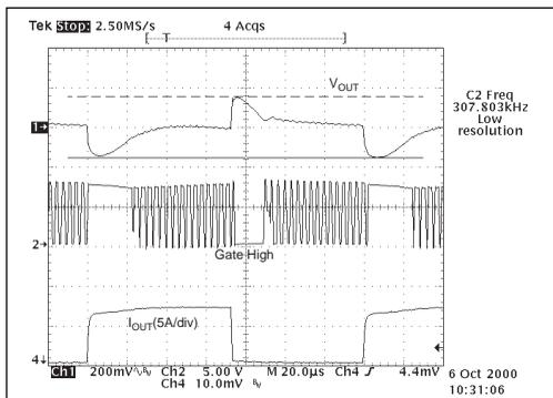
Figure 5. Load Step Response: 0.4A to 7A
