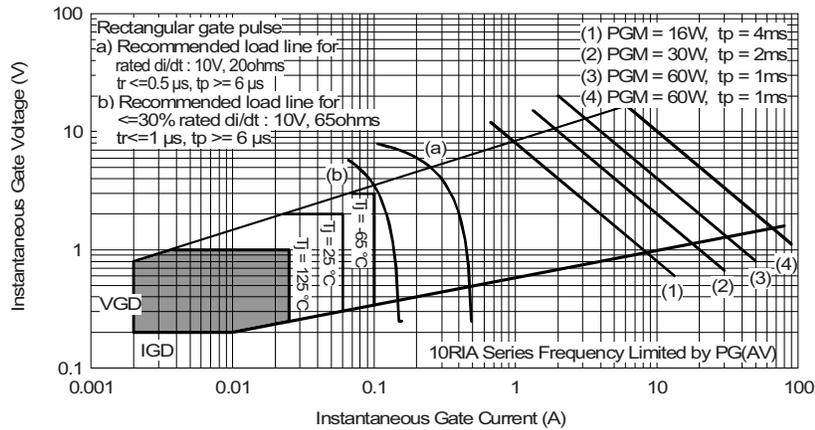
Fig. 9 - Gate Characteristics
