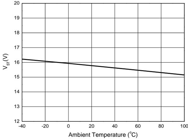
**Shutdown Voltage vs. Ambient Temperature**
