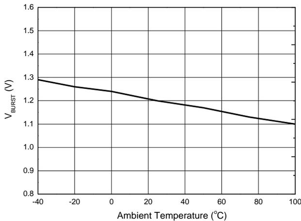
**V<sub>BR-IN</sub> vs. Ambient Temperature**
