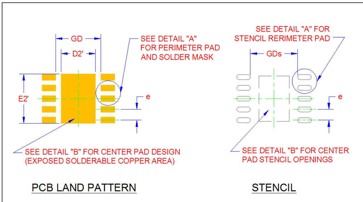
FIGURE 6-4: CAP1206 PCB DETAIL A - 10-PIN DFN 3MM X 3MM
