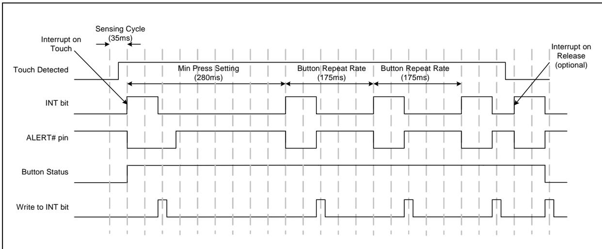
**FIGURE 4-4: SENSOR INTERRUPT BEHAVIOR - NO REPEAT RATE ENABLED**
