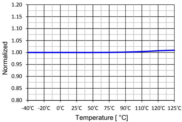
Figure 13. Shutdown Feedback Voltage ( $V_{\text{SD}}$ ) vs.  $T_A$
