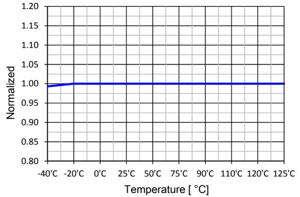
Figure 12. UVLO Threshold Voltage ( $V_{\text{STOP}}$ ) vs.  $T_A$
