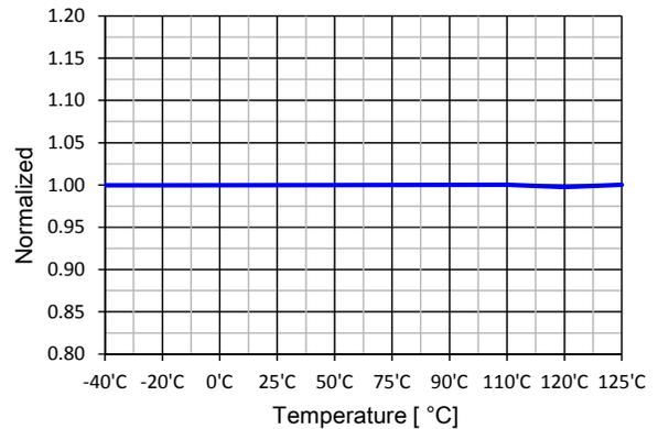
Figure 16. Maximum Duty Ratio ( $D_{\text{MAX}}$ ) vs.  $T_A$
