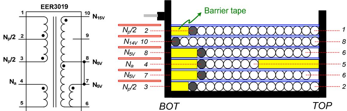
Figure 26. Transformer Specification
