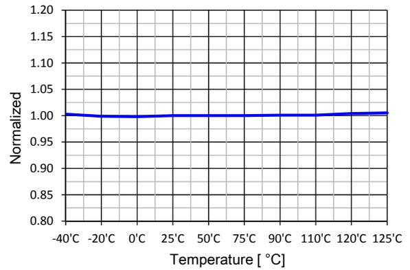
Figure 14. Over-Voltage Protection ( $V_{\text{OVP}}$ ) vs.  $T_A$
