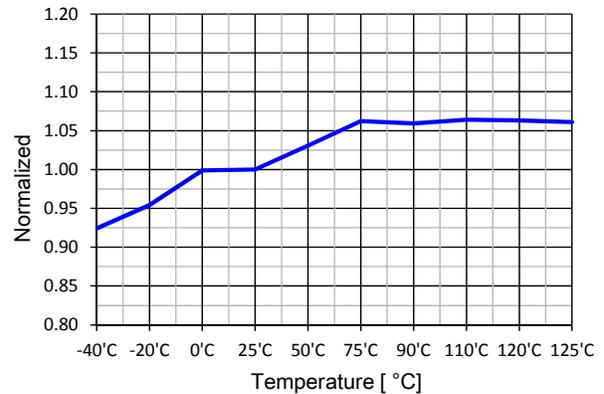
**Figure 10. Shutdown Delay Current ( $I_{DELAY}$ ) vs.  $T_A$**
