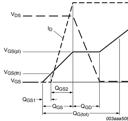
Fig. 15. MOSFET transistor: Gate charge waveform definitions
