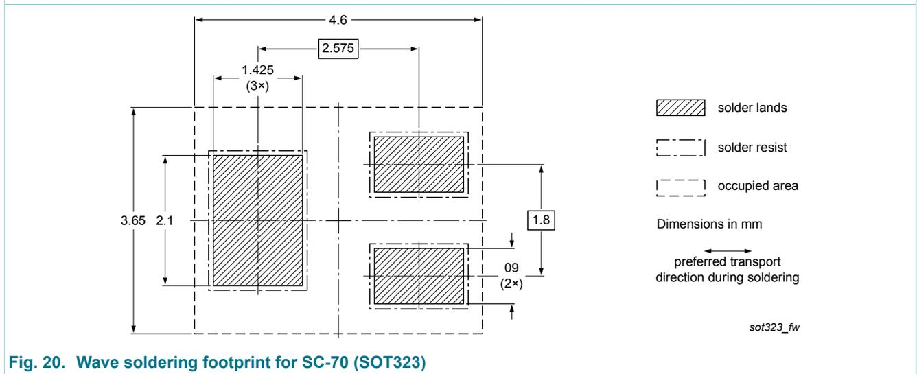
Fig. 20. Wave soldering footprint for SC-70 (SOT323)
