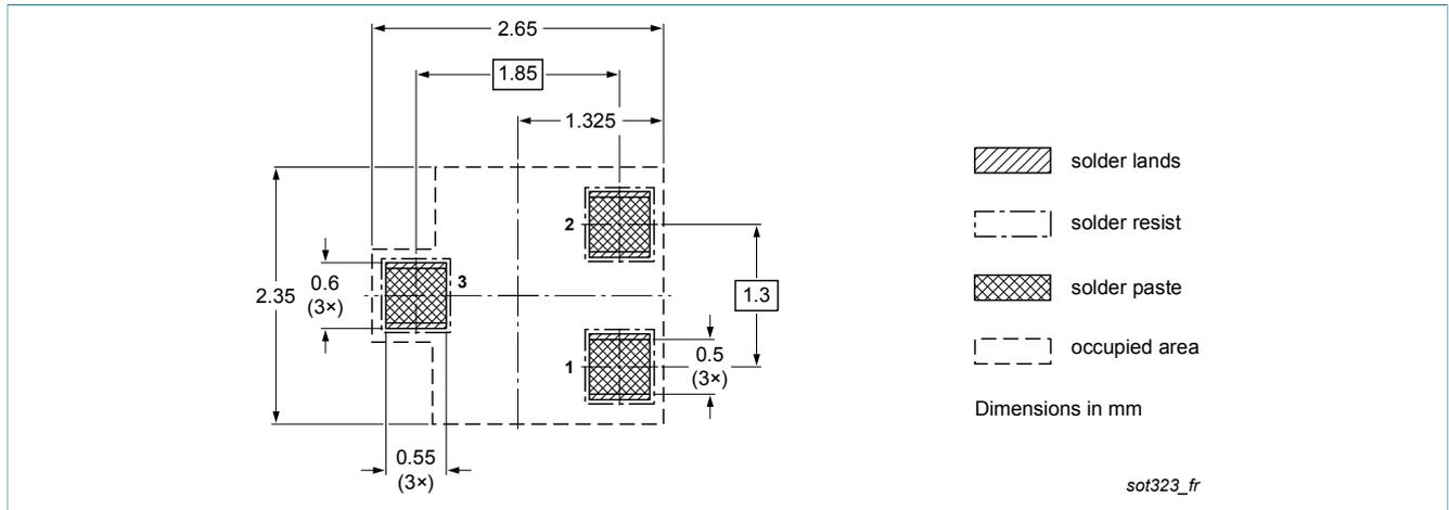
Fig. 19. Reflow soldering footprint for SC-70 (SOT323)
