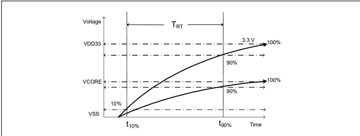
**Note:** The Power Supply Rise time requirement does not apply if the **RESET\_N** signal is held low during power on and released after power levels rise and stabilize above the power on thresholds, or if the **RESET\_N** signal is toggled after power supplies become stable.
