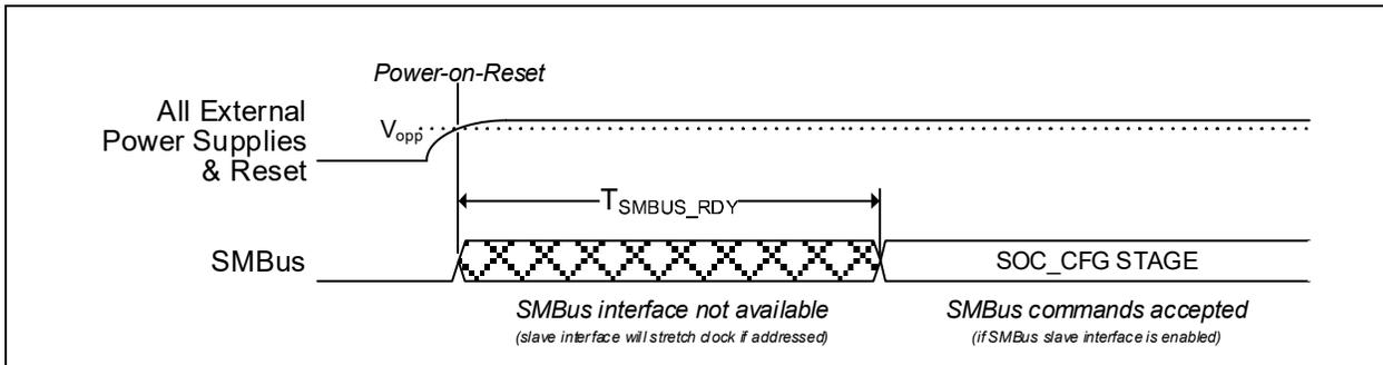
**TABLE 9-7: POWER-ON OR RESET TO SMBUS SLAVE READY TIMING**
