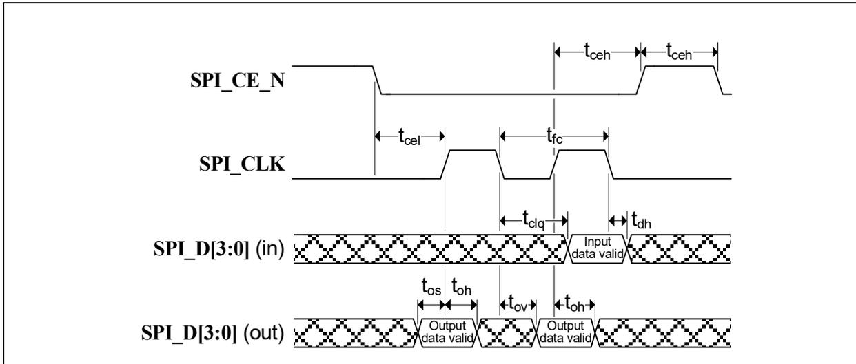
**TABLE 9-9: SPI/SQI MASTER TIMING (30 MHZ OPERATION)**
