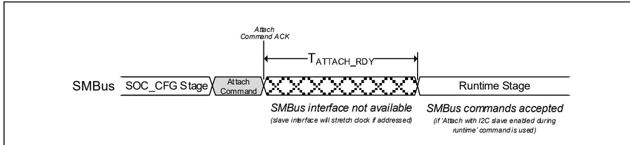
**TABLE 9-8: USB ATTACH COMMAND TO SMBUS SLAVE READY TIMING**
