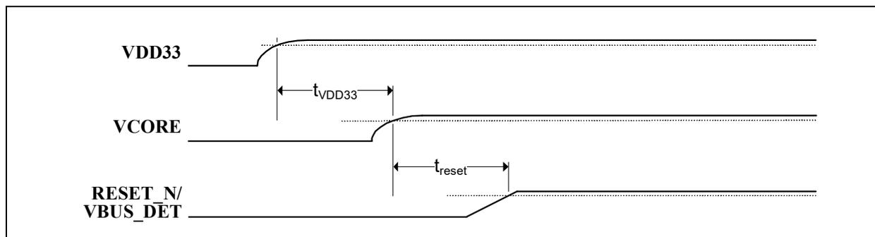
**TABLE 9-4: POWER SUPPLY AND RESET\_N SEQUENCE TIMING**
