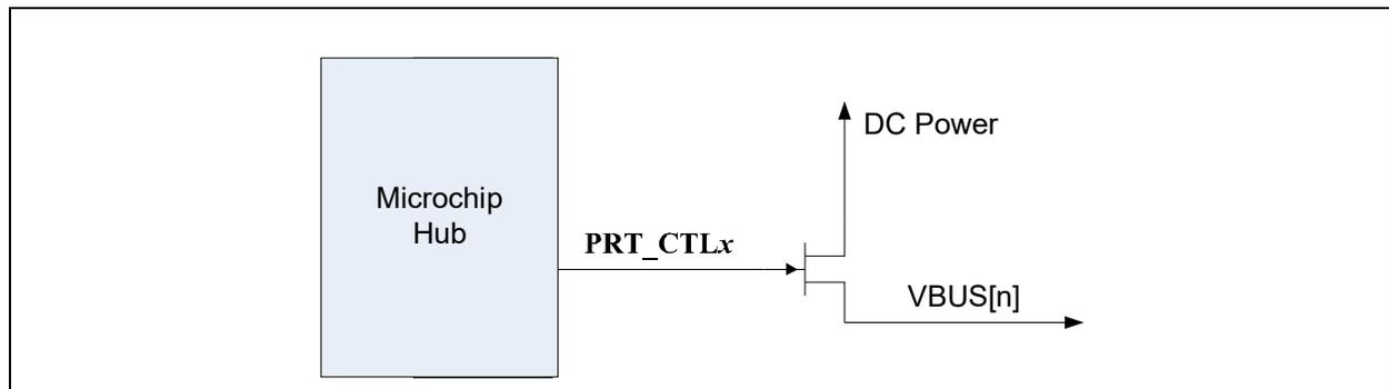
If the OEM provides an external supply capable of supplying current per the battery charging specification, the hub can be configured to indicate the presence of such a supply from the device. This indication, via the **PRT\_CTLx** pins, is on a per port basis. For example, the OEM can configure two ports to support battery charging through high current power FETs and leave the other two ports as standard USB ports.
