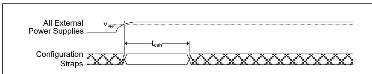
**TABLE 9-5: POWER-ON CONFIGURATION STRAP LATCHING TIMING**
