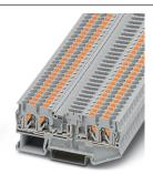
Disconnect terminal block, nom. voltage: 400 V, nominal current: 20 A, connection method: Push-in connection, cross section: 0.14 mm² - 4 mm², AWG: 26 - 12, length: 79.6 mm, width: 5.2 mm, color: gray, mounting: NS 35/7,5, NS 35/15
