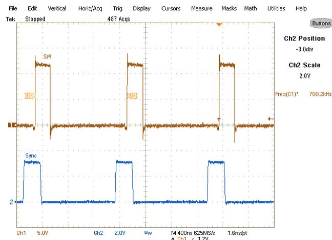
Fig. 26: Synchronization to 700kHz external clock signal at 9A load
