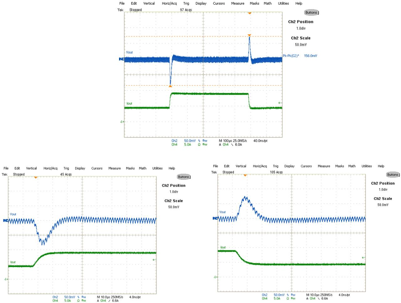
Fig. 24: Transient Response, 4.5A to 9A step 2.5A/ $\mu$ s
