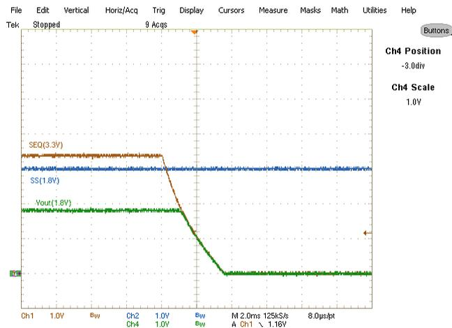
Fig. 27: Simultaneous Tracking a 3.3V input at power-up and shut-down
