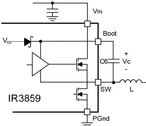
Fig. 13. Bootstrap circuit to generate Vc voltage
