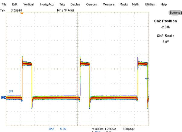
Fig. 22: Inductor node at 9A load
