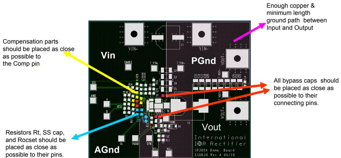
Fig. 28a. IRDC3859 demoboard layout considerations – Top Layer
