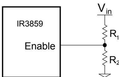
For a maximum Enable threshold of  $V_{EN} = 1.36\text{ V}$
