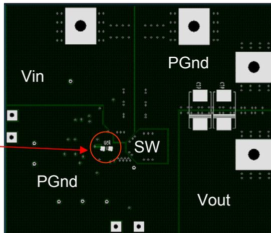
Fig. 28b. IRDC3859 demoboard layout considerations – Bottom Layer
