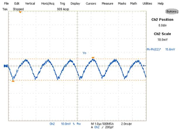
Fig. 21: Output Voltage Ripple, 9A load Ch<sub>2</sub>: V<sub>out</sub>
