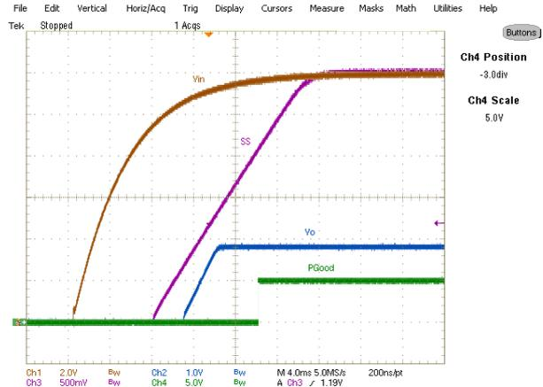
Fig. 19: Start up at 9A Load,
