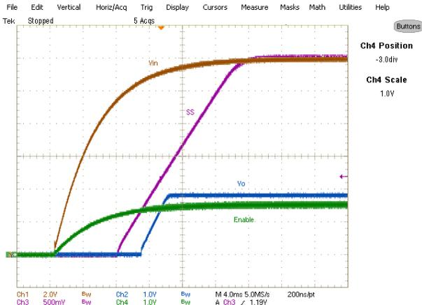
Fig. 18: Start up at 9A Load
