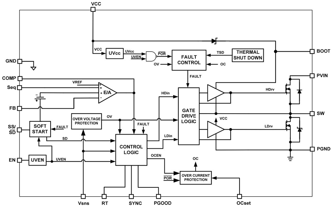
Fig. 2. Simplified block diagram of the IR3859
