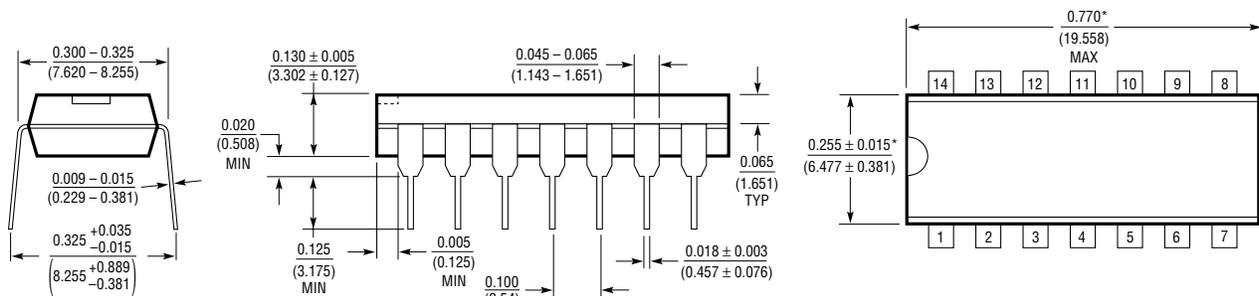
\*THESE DIMENSIONS DO NOT INCLUDE MOLD FLASH OR PROTRUSIONS.
