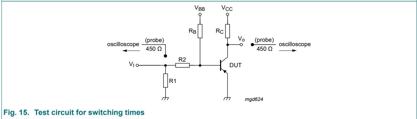
Fig. 15. Test circuit for switching times
