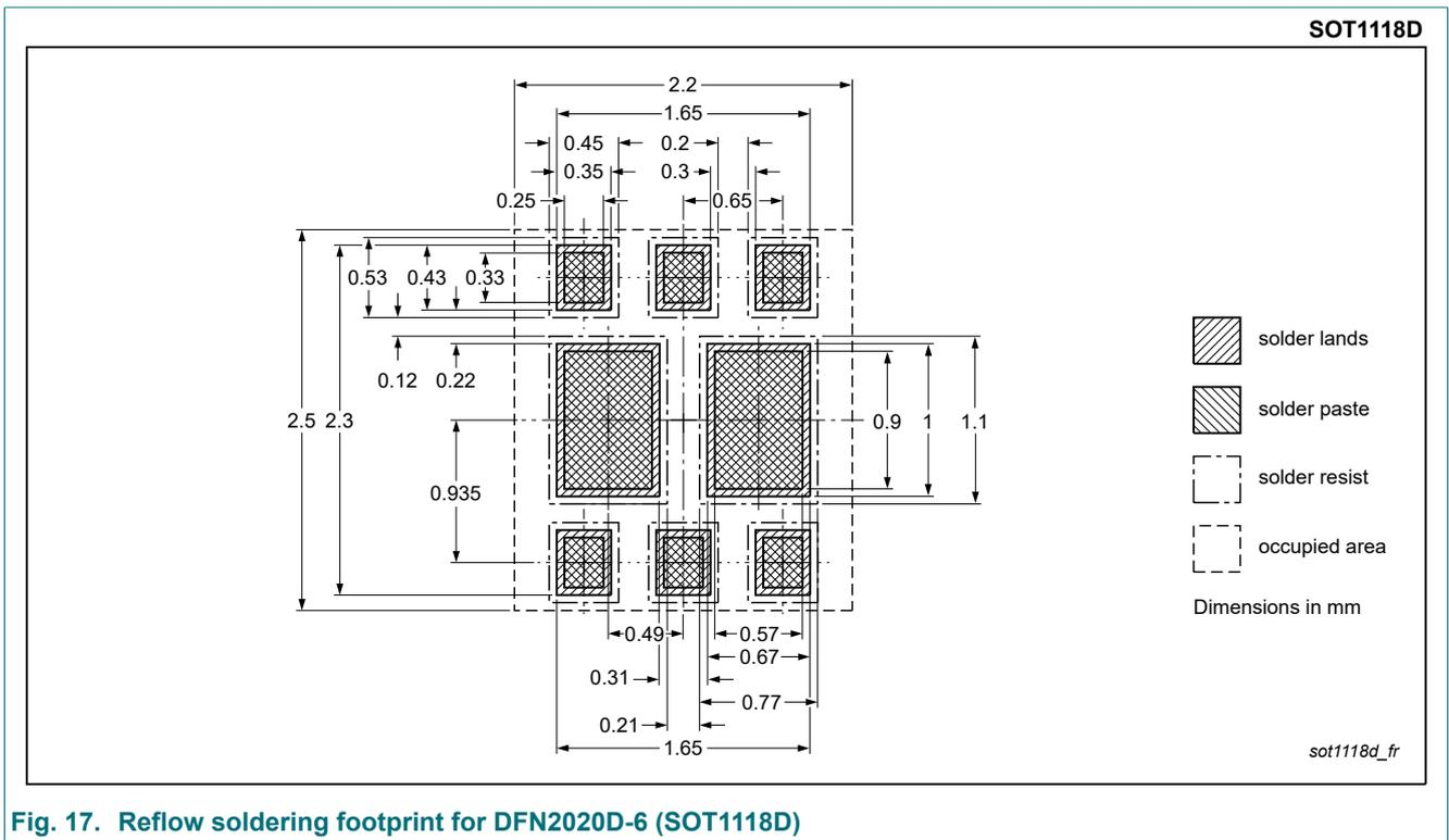
Fig. 17. Reflow soldering footprint for DFN2020D-6 (SOT1118D)
