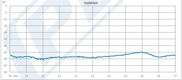
Click the following link (or enter part number in "SEARCH" on website) to obtain additional part information including price, inventory and certifications: Dual Junction Isolator With 34 dB Isolation From 18 GHz to 26.5 GHz, 5 Watts And SMA Female PE83IR1025
