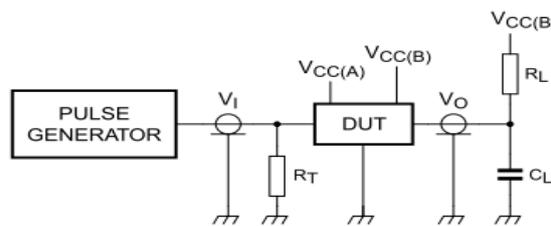
R<sub>L</sub> = Load resistor: 1.35kΩ on port B; 167Ω on port A (0.8V to 2.7V) and 450Ω on port A (3.0V to 5.5V)
