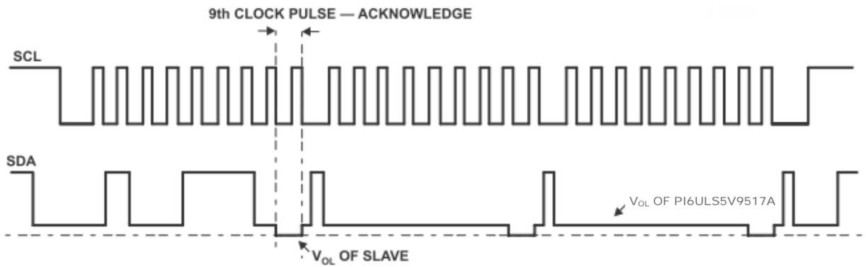
Figure 10: Bus B (2.2V to 5.5V Bus) Waveform
