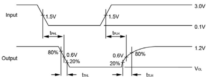
Figure 2: Propagation Delay and Transition Times B→A
