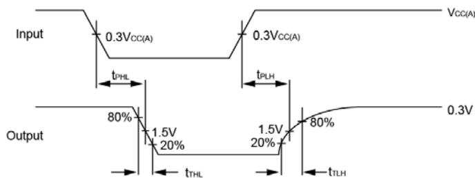
Figure 3: Propagation Delay and Transition Times A→B
