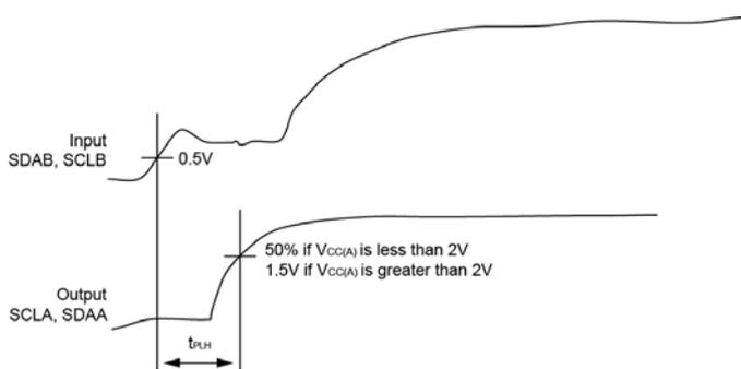
Figure 4: Propagation Delay
