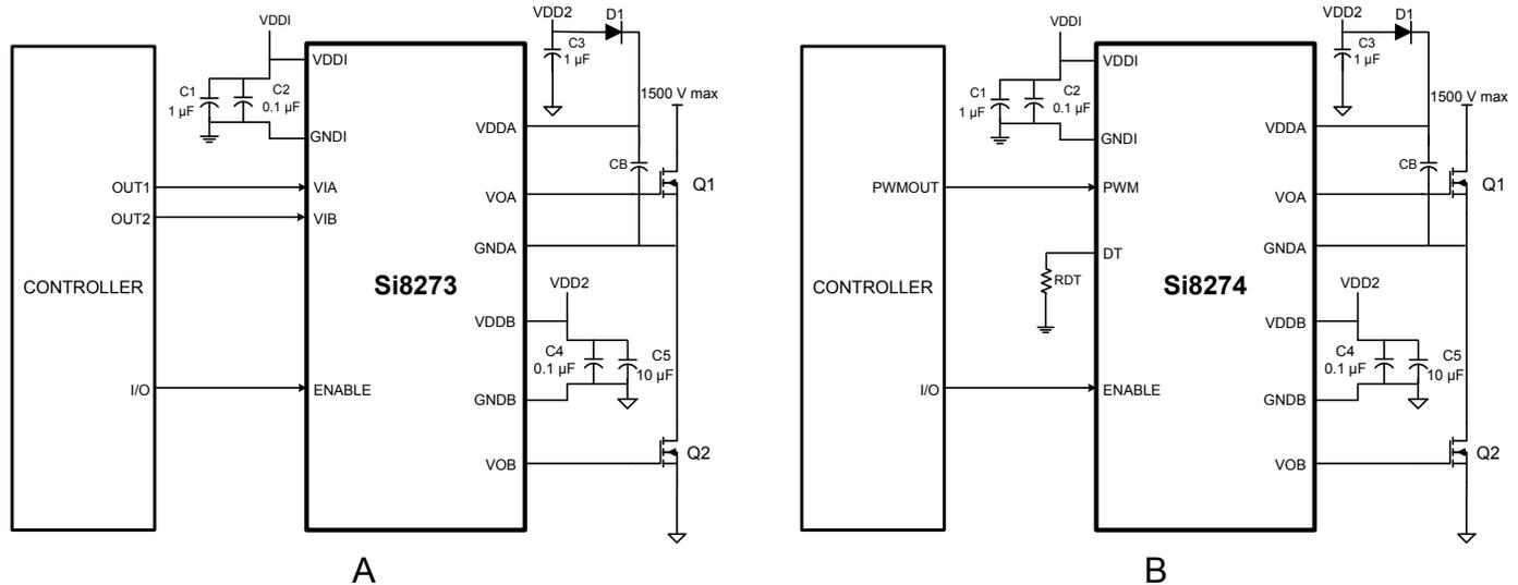
**Figure 3.1. Si827x in Half-Bridge Application**
