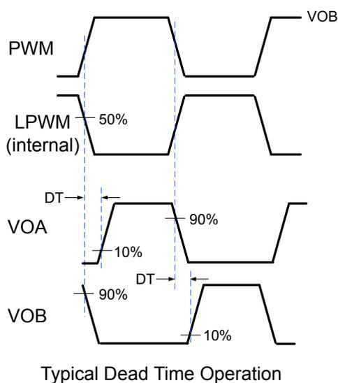
**Figure 2.20. Dead Time Waveforms for Si8274 Drivers**
