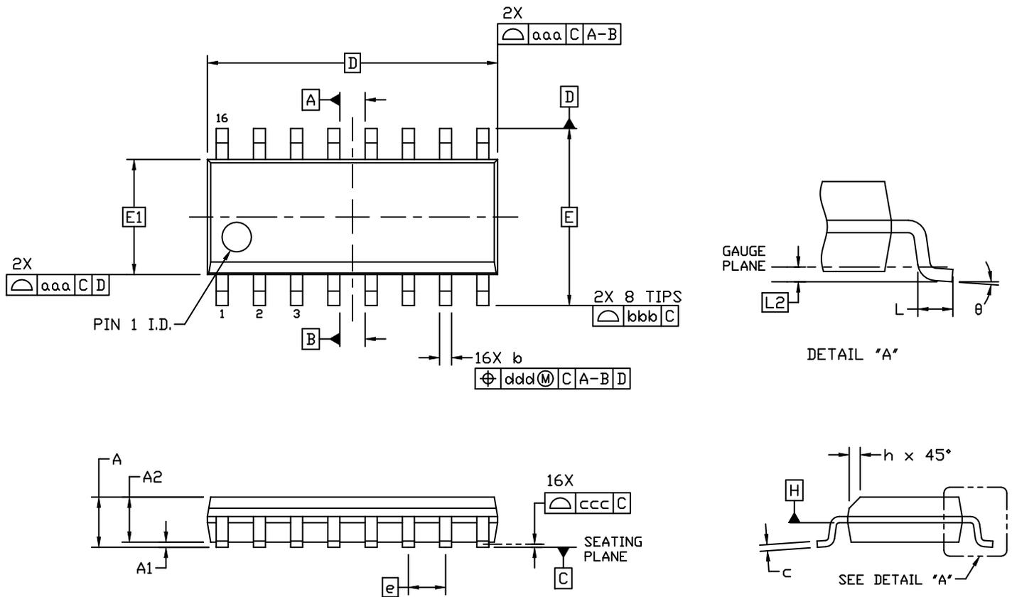
Figure 6.1. 16-pin Small Outline Integrated Circuit (SOIC) Package
