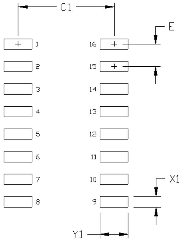
Figure 7.1. 16-Pin Narrow Body SOIC PCB Land Pattern
