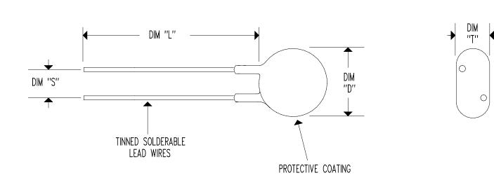
RESISTANCE @  $+25^{\circ}C = 8~\Omega~\pm~20\%$  MAXIMUM STEADY STATE CURRENT = 1 AMP RESISTANCE @ MAXIMUM CURRENT = 0.50  $\Omega$  NOMINAL
