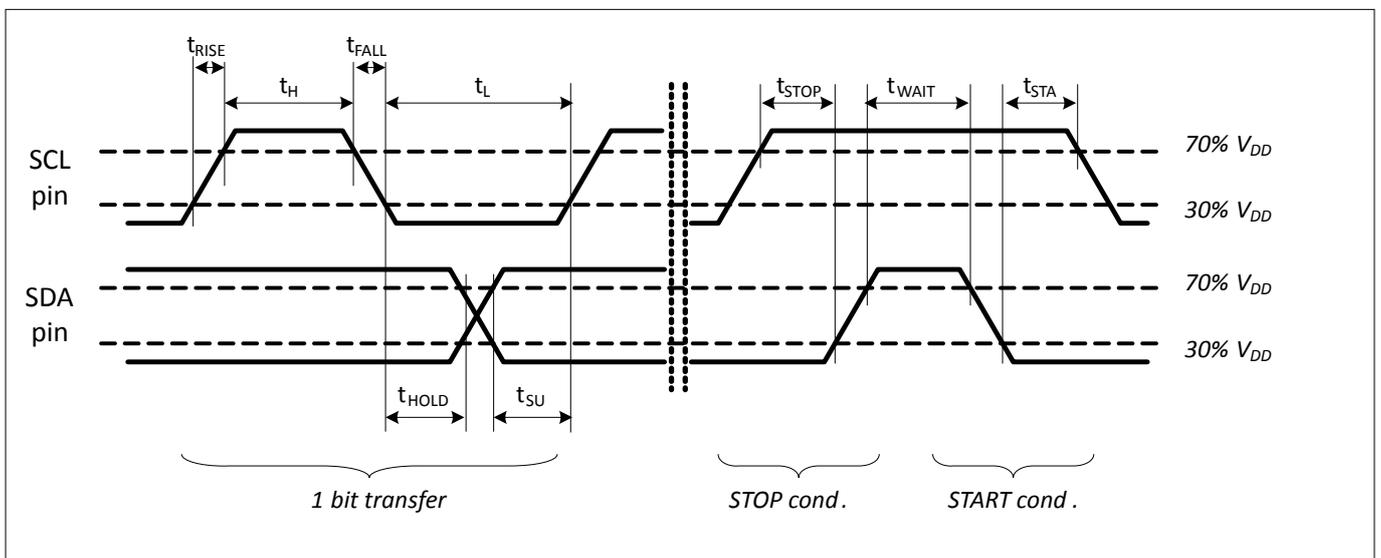
**Figure 9** I<sup>2</sup>C timing specification
