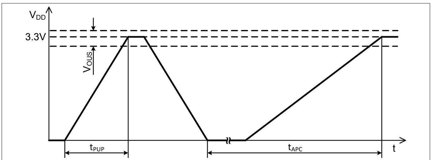
Figure 7 V<sub>DD</sub> power up and power cycle for high availability
