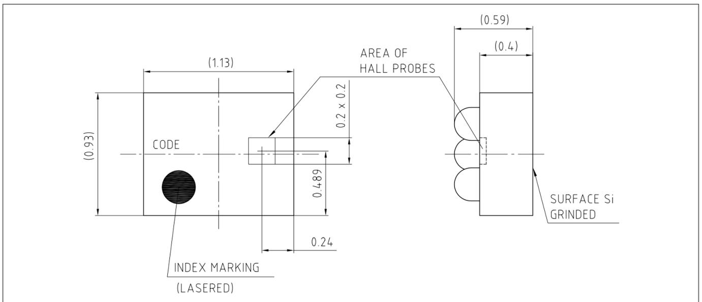
**Figure 4** Center of sensitive area (dimensions in mm)
