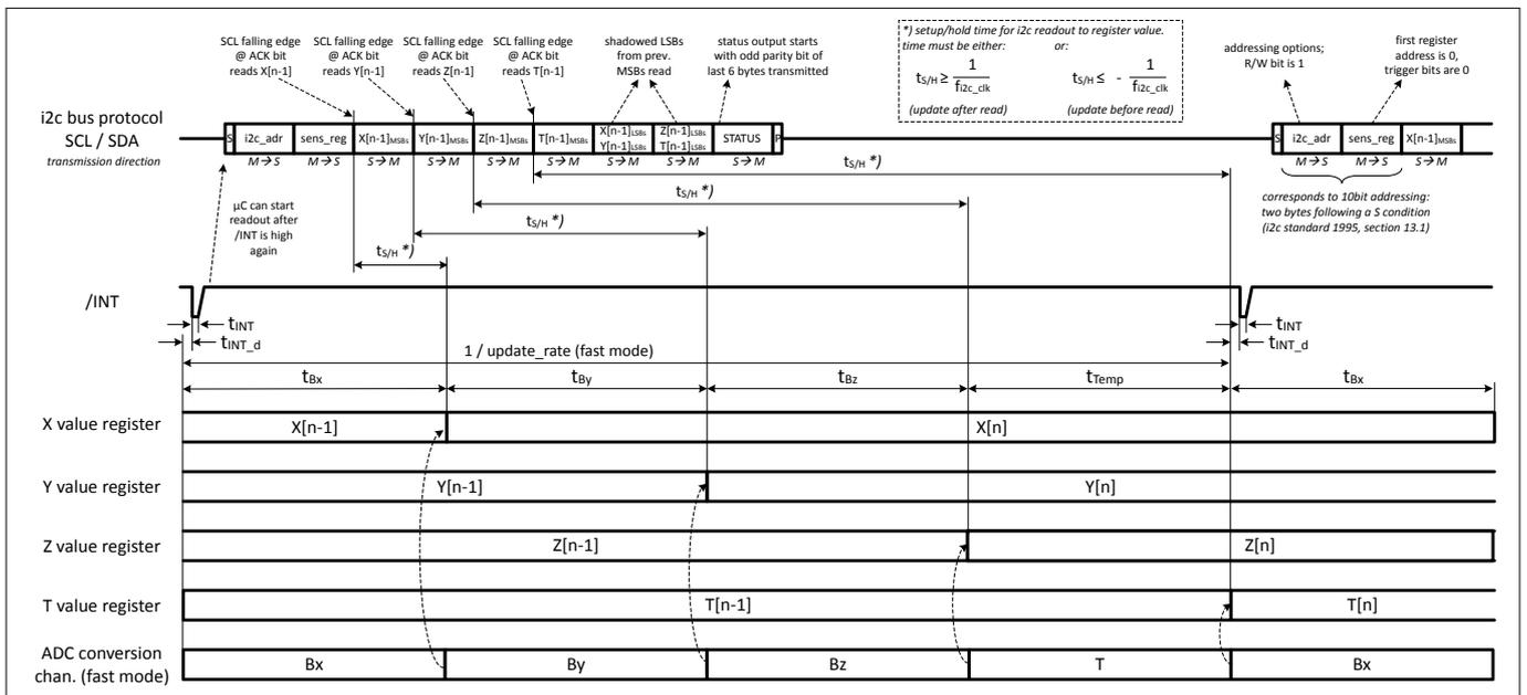
**Figure 8** I<sup>2</sup>C readout frame, ADC conversion and related timing
