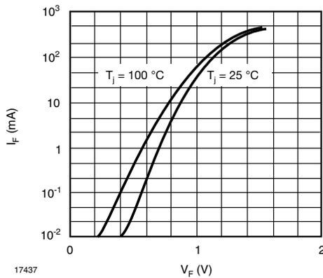
Fig. 1 - Forward Characteristics
