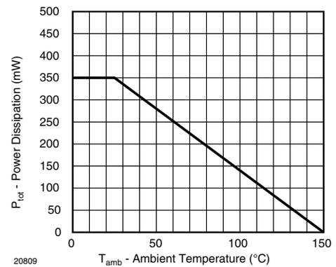
Fig. 3 - Admissible Power Dissipation vs. Ambient Temperature
