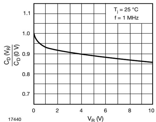
Fig. 4 - Relative Capacitance vs. Reverse Voltage
