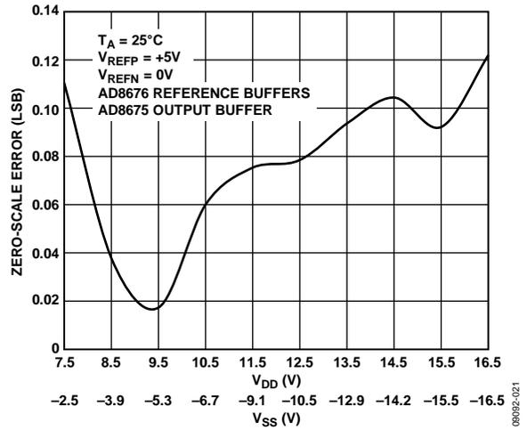
Figure 20. Zero-Scale Error vs. Supply Voltage, +5 V Span
