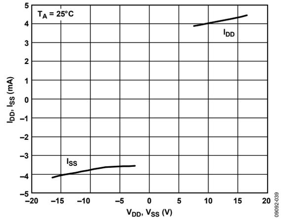
Figure 38. Power Supply Currents vs. Power Supply Voltages
