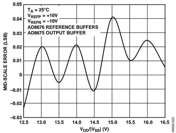
Figure 21. Midscale Error vs. Supply Voltage, ±10 V Span
