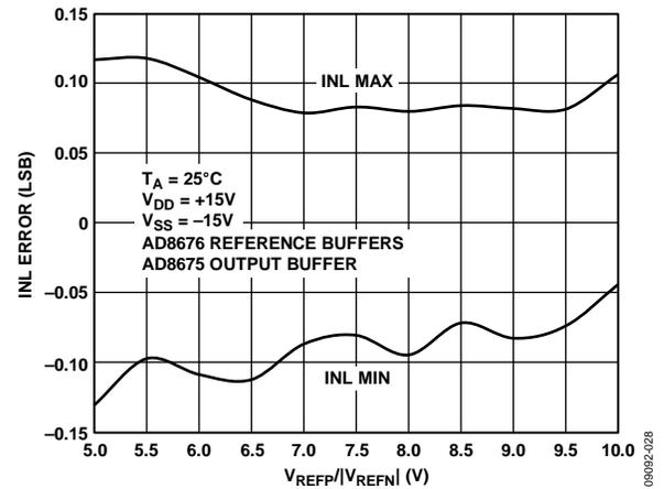
Figure 27. Integral Nonlinearity Error vs. Reference Voltage
