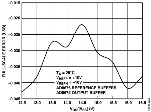
Figure 23. Full-Scale Error vs. Supply Voltage, ±10 V Span
