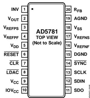
Figure 4. Pin Configuration
