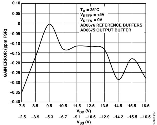
Figure 26. Gain Error vs. Supply Voltage, +5 V Span
