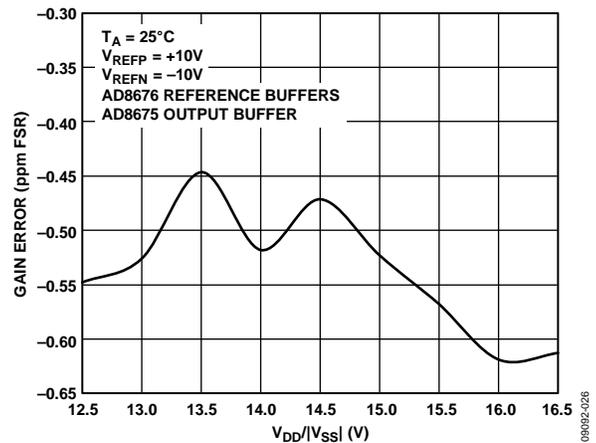
Figure 25. Gain Error vs. Supply Voltage, ±10 V Span
