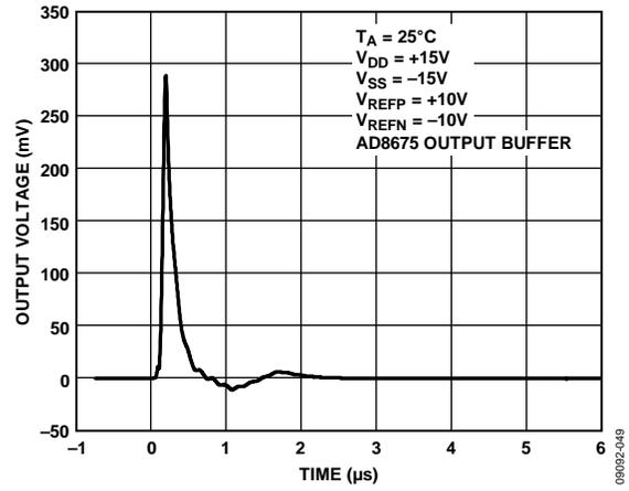
Figure 48. Glitch Impulse on Removal of Output Clamp
