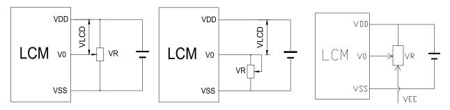
V<sub>DD∼</sub>V₀: LCD Driving voltage VR: 10k~20k
