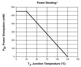
\*FR-5 board (1.0 x 0.75 x 0.062in) with copper mounting pad area of 2.9mm  $^{\!2}$
