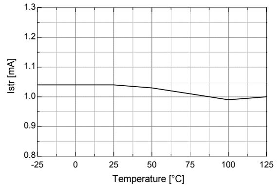
Figure 9. V<sub>STR</sub> Star-up Current vs. Temp.
