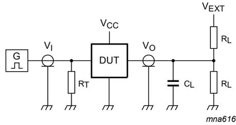
Test data is given in [Table 9](#). Definitions for test circuit:
