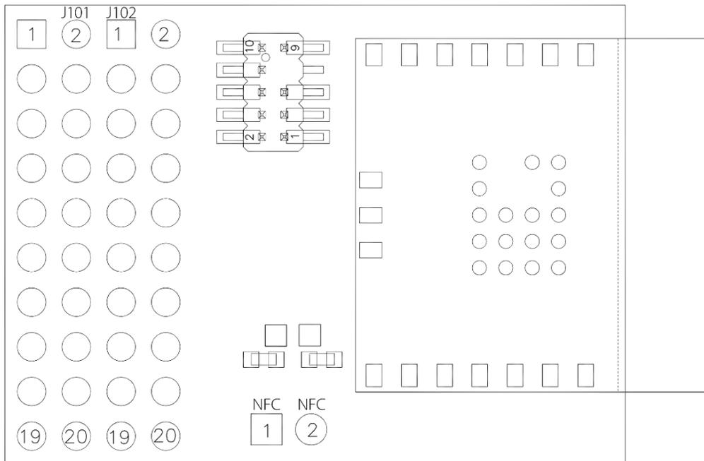
Figure 8: D52Q M6 (Development Module) - Top View
