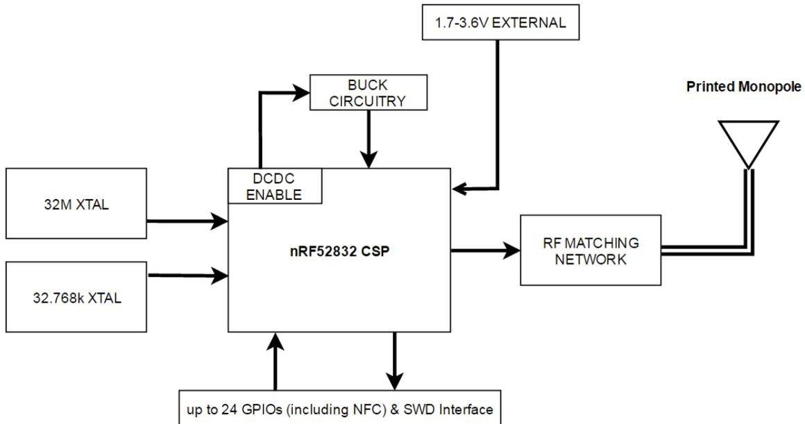
Figure 5: D52MD2M8IA, D52MPMM8IA Models Module Block Diagram
