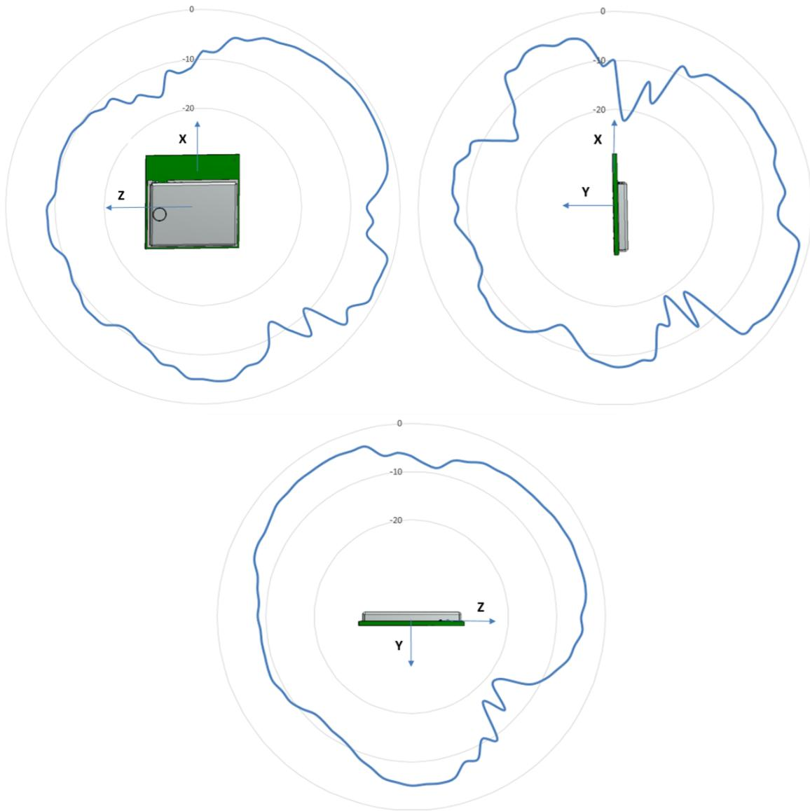
**Figure 17: D52Q M4 Module Typical Antenna Gain (dBi)**
