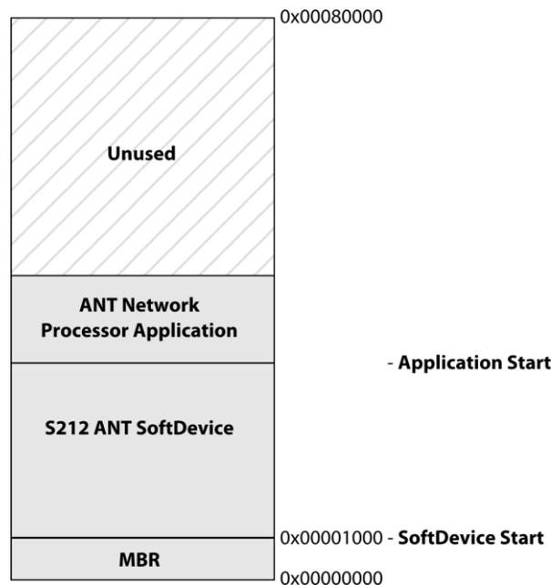
**Figure 10: Memory Map of the Preloaded Software**
