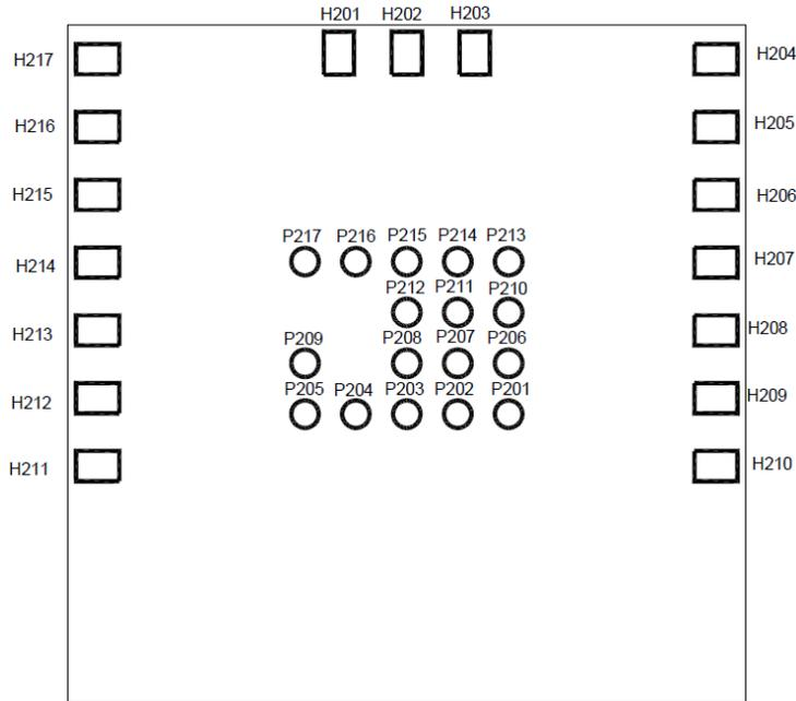
Figure 6: D52Q M4 (20mm x 20mm) Bottom View
