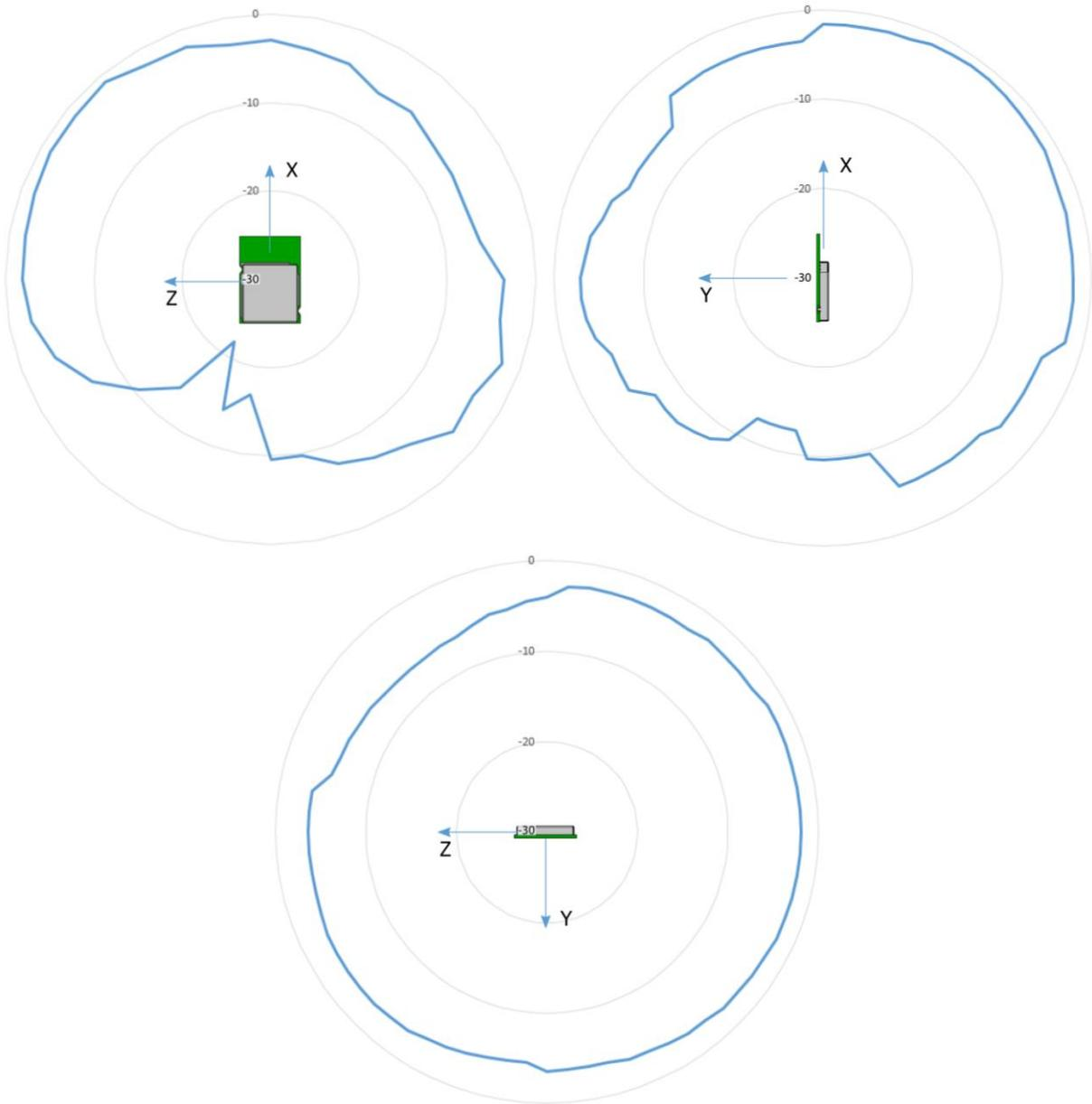
Figure 18: D52M M8 Module Typical Antenna Gain (dBi)
