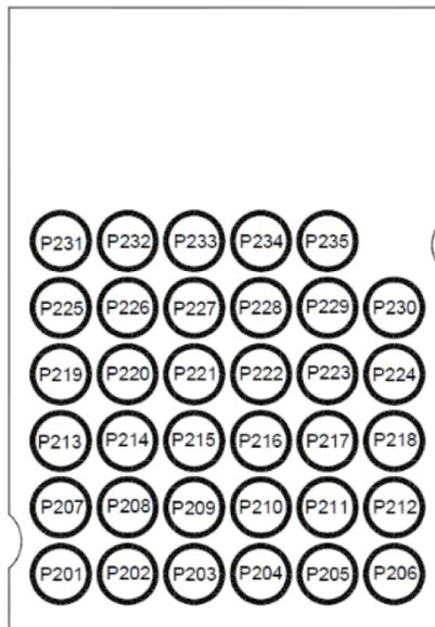
Figure 7: D52M M8 (14.0mm x 9.8mm) Bottom View
