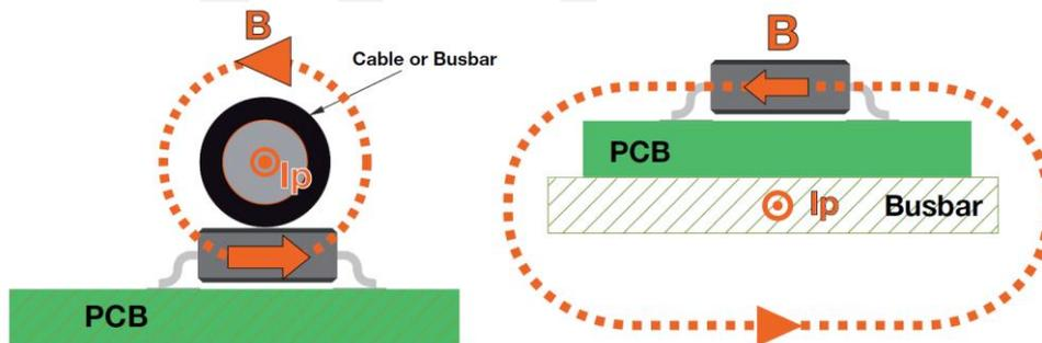
Figure X Example with cable or busbar
