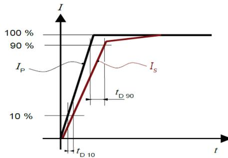
Figure X  $t_{D10}$  (delay time @ 10 %) and  $t_{D90}$  (delay time @ 90 %).
