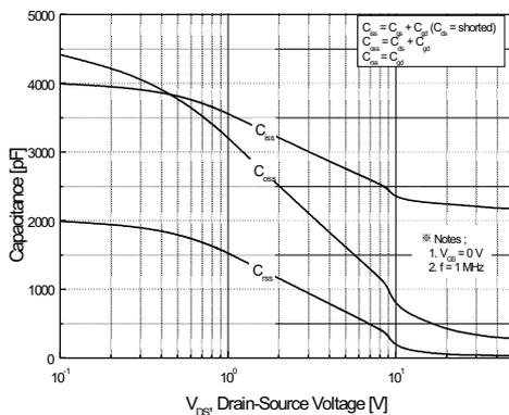
Figure 5. Capacitance Characteristics
