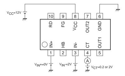
CT pin charge/discharge voltage (VCT)
