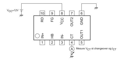
OUT output saturation voltage ( $V_{OL}$ ,  $V_{OH}$ )
