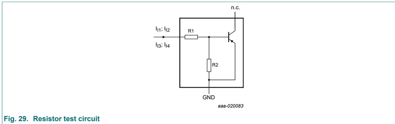
Fig. 29. Resistor test circuit
