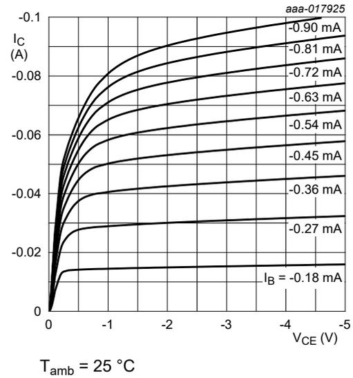
**Fig. 5. PDTA143EQB: Collector current as a function of collector-emitter voltage; typical values**
