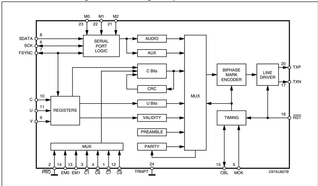
Figure 9. Block diagram - consumer mode
